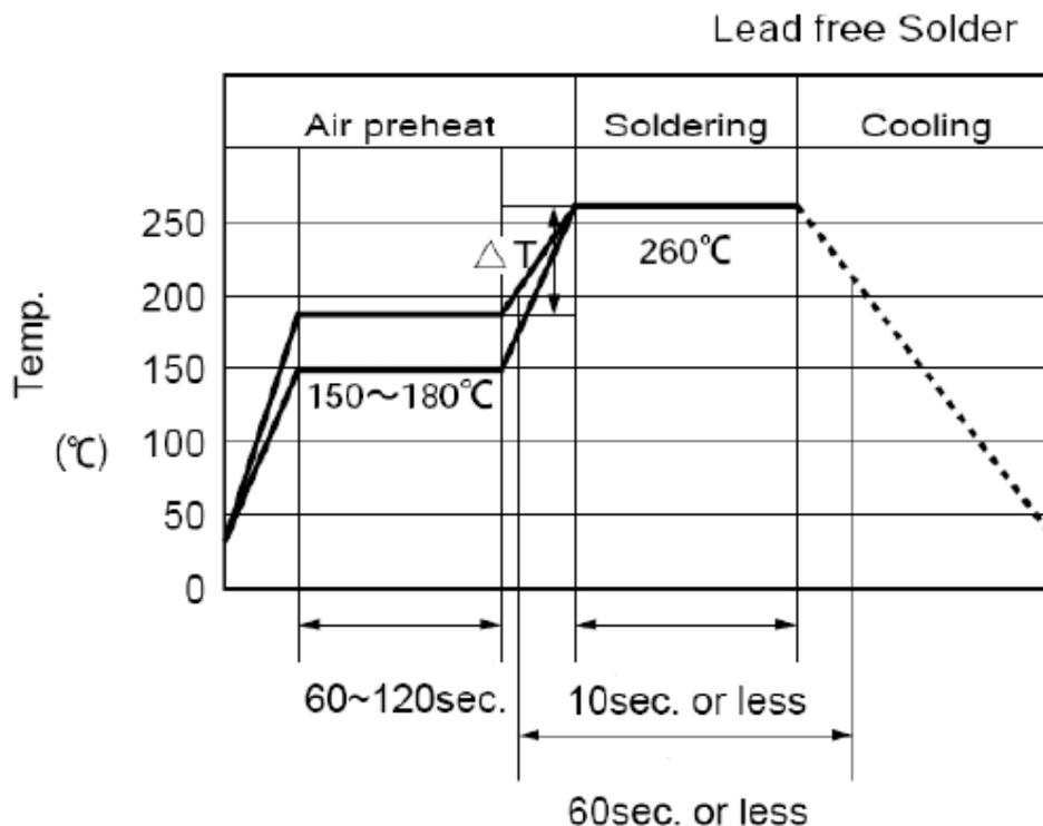
1. Time shown in the above figures is measured from the point when chip surface reaches temperature.
