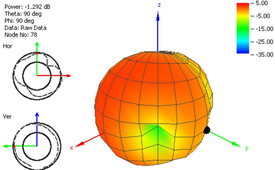
Figure 8. Radiation Pattern at 2400 MHz of the SDWA.01 antenna.
