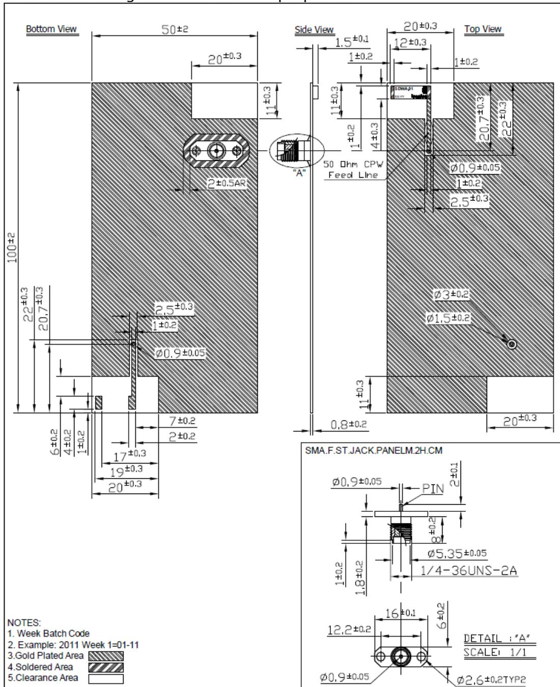
The size of the ground plane for the complete evaluation board is 100x50 mm. The area occupied by the antenna is 20x11mm.
