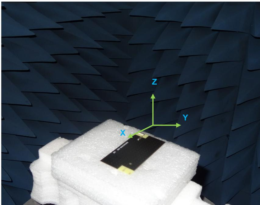
Figure 2. Peak gain, efficiency, and radiation pattern measurement
