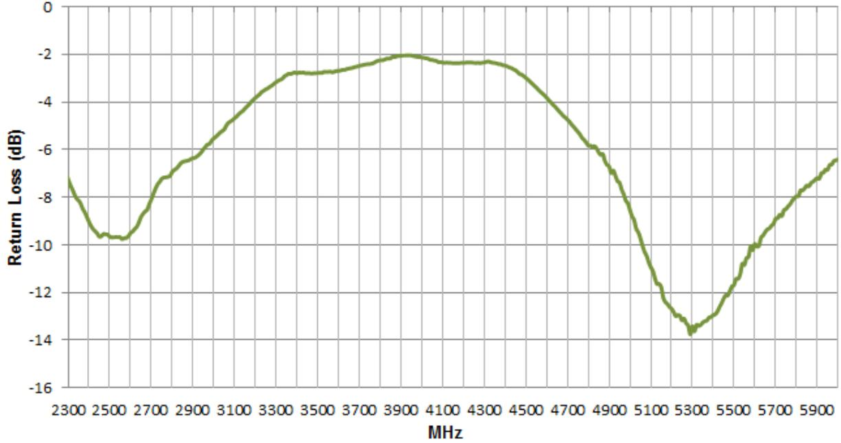
Figure 3. Return Loss of the SDWA.01 antenna.
