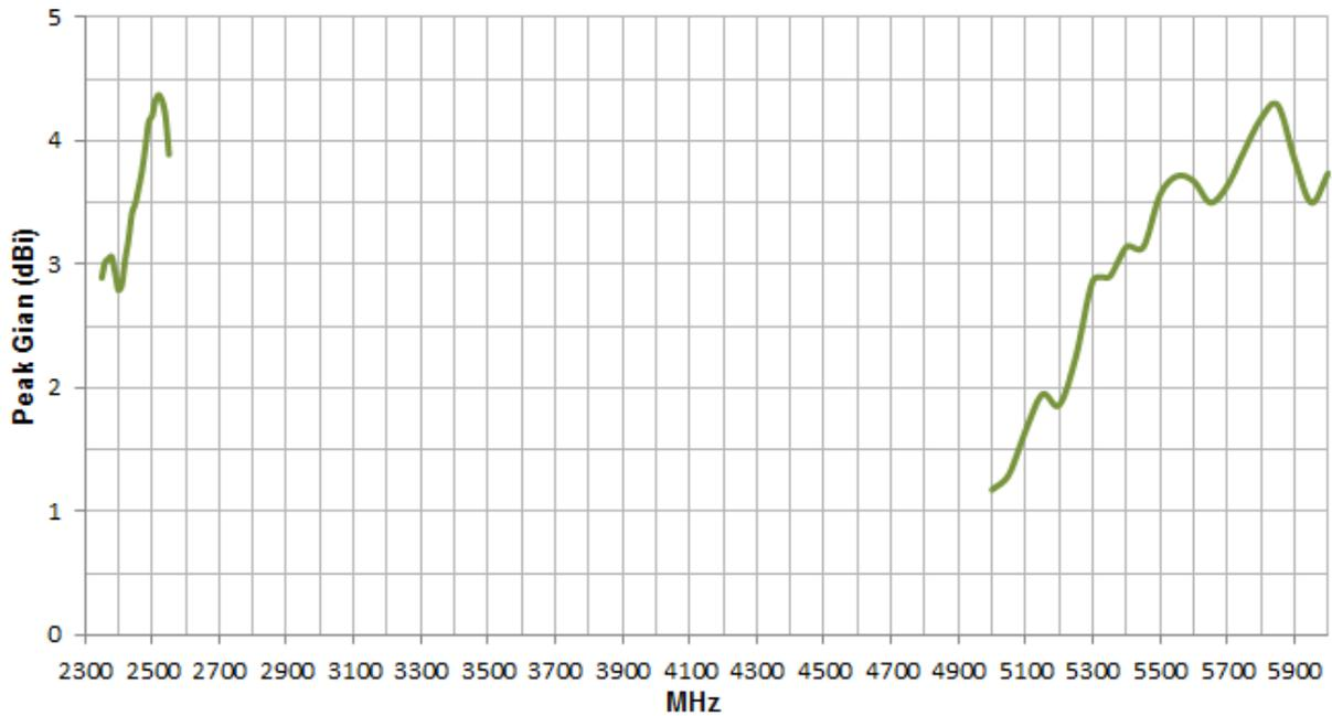
Figure 6. Peak gain of the SDWA.01 antenna.
