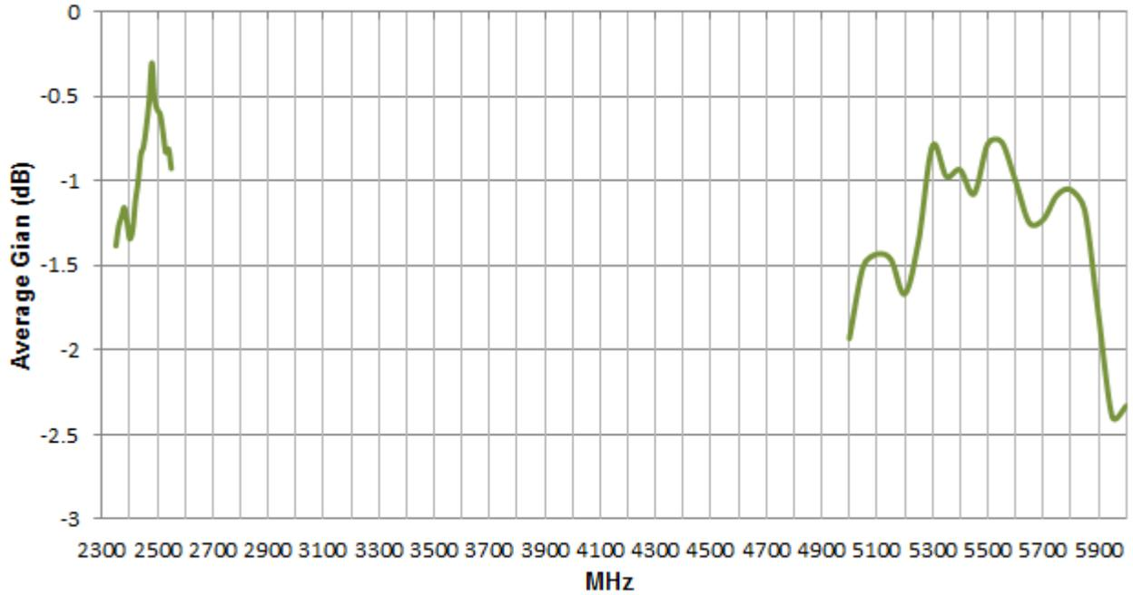
Figure 7. Average gain of the SDWA.01 antenna.
