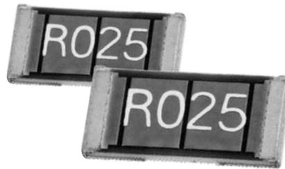
Ohmite's LVC Series low value chip resistors are ideal for today's current sense applications requiring low profile, low cost solutions. Available in 0.5, 0.75, and 1 watt sizes, footprints are 1206, 2010, and 2512 size respectively. These resistors are offered in ohmic ranges from 0.10 to 4.7 ohms in standard 1% and 2% in E12 values depending on value.
