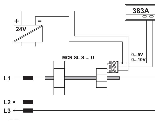
Figure 1 Current measurement
