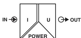
The **MCR-SL-S...-I-LP** current measuring transducers convert sinusoidal and non-sinusoidal alternating currents up to 400 A into the analog standard signal of 4...20 mA. The measuring range at the output is set with a switch. On the output side, the current measuring transducers are operated in a 4...20 mA current loop, which simultaneously provides the power supply for the modules, which is necessary for signal conversion.
