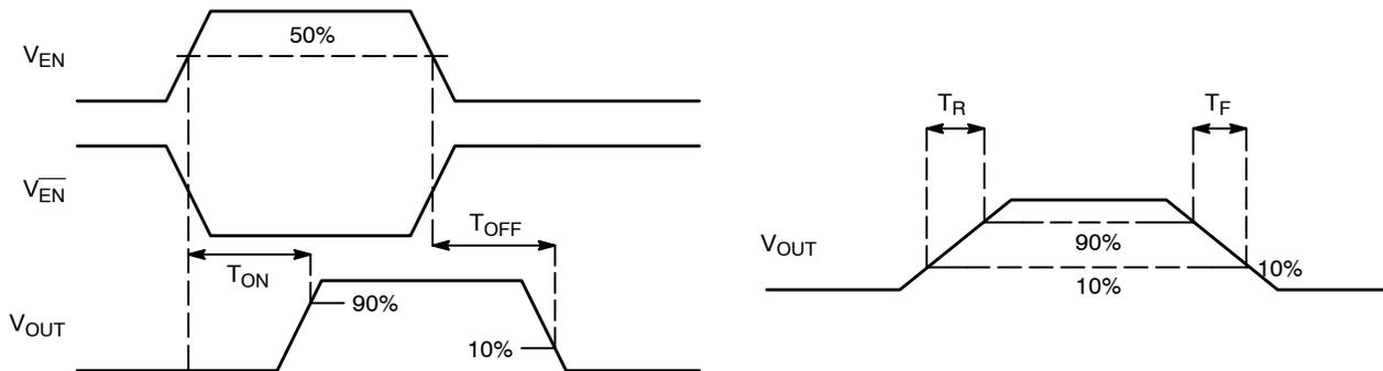
**Figure 4. Voltage Waveform**
