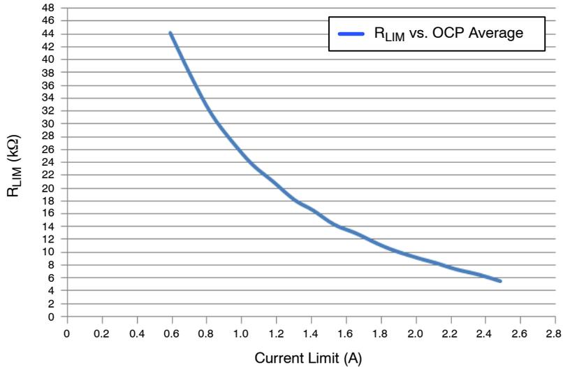
**Figure 25. R<sub>LIM</sub> Curve vs. Current Limit**
