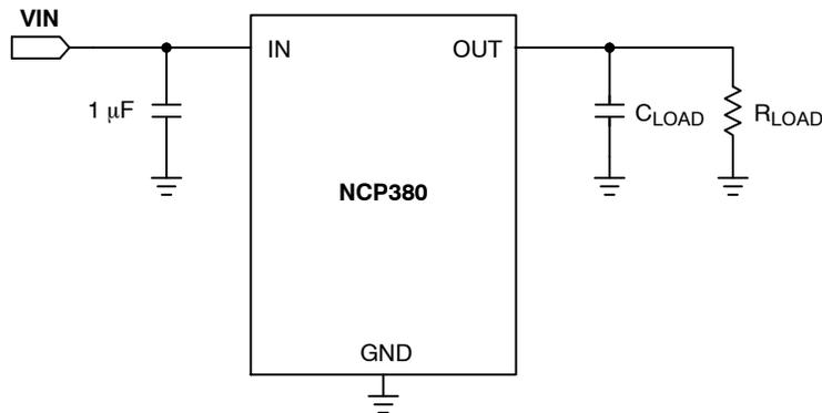
**Figure 3. Test Configuration**
