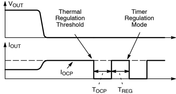
Figure 24. Short circuit
