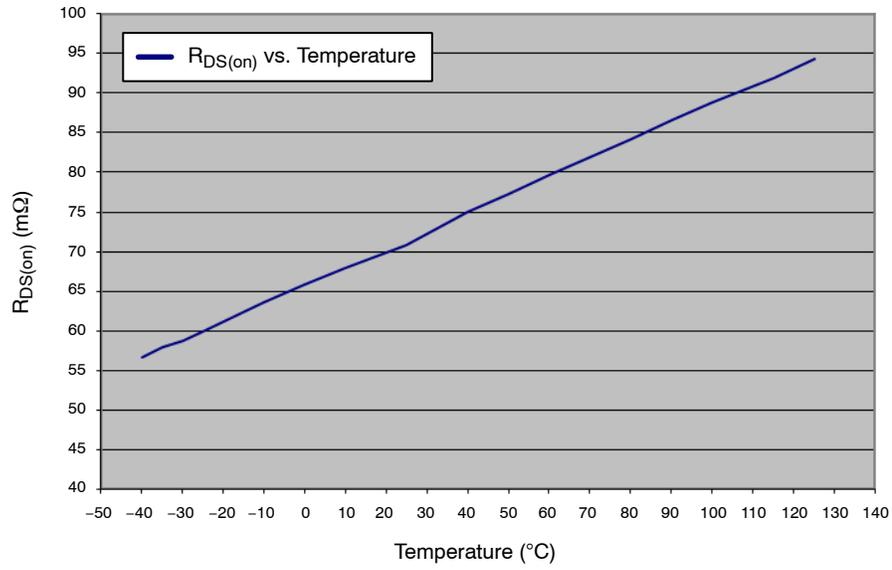
Figure 20. R<sub>DS(on)</sub> vs Temperature, TSOP Package
