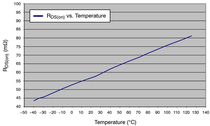
Figure 21. R<sub>DS(on)</sub> vs Temperature, μDFN Package
