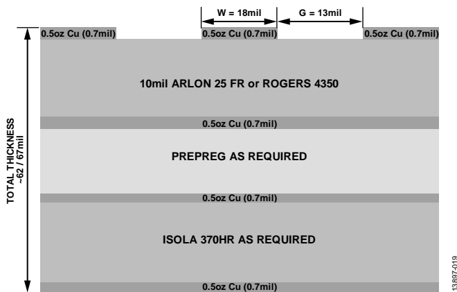
Figure 94. Evaluation Board Cross Sectional View
