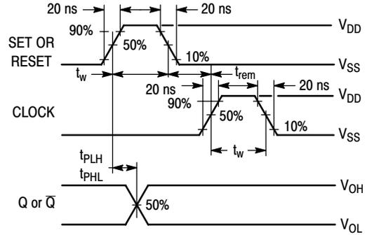
**Figure 2. Dynamic Signal Waveforms
