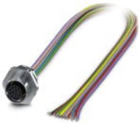
Flush-type connector, Universal, 12-position, SocketLink:M12, A-coded, Front mounting, M16 x 1.5, Individual wires, Cable length: 0.5 m
