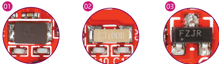
Figure 5-1: Crystal oscillator and 2.048V reference
