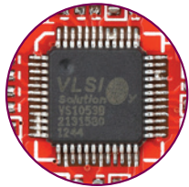
Figure 9-1: On-board VS1053 MP3 codec
