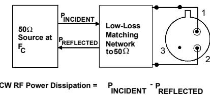
$$CW \text{ RF Power Dissipation} = P_{\text{INCIDENT}} - P_{\text{REFLECTED}}$$
