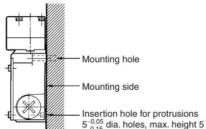
The D4BS can be mounted more securely by adding two protruding portions, each of which is 5 mm maximum in height and  $5^{-0.05}_{+0.15}$  mm in diameter as shown below.
