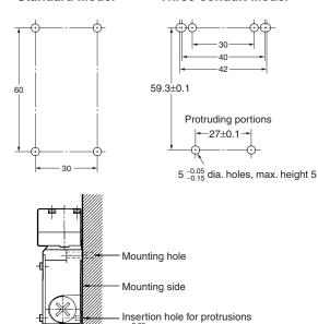
The D4BS can be mounted more securely by adding two protruding portions, each of which is 5 mm maximum in height and 5  $^{-0.05}/_{-0.15}$  mm in diameter as shown below.
