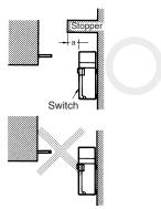
Refer to *Dimensions* for the mounting dimension of the Operation Key and mount the Operation Key correctly. The Operation Key will soon become damaged or worn out if it is not mounted correctly.
