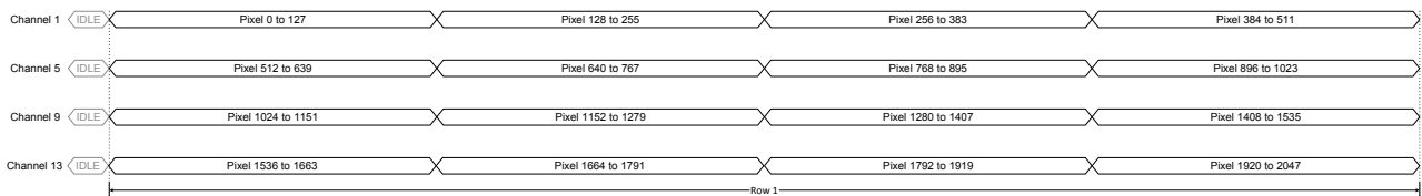
Figure 28: Pixel remapping for 4 output channels
