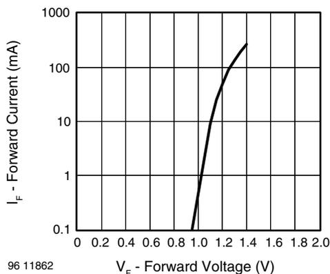
Fig. 7 - Forward Current vs. Forward Voltage
