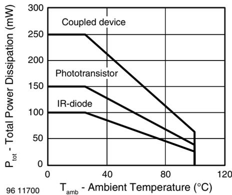
Fig. 6 - Total Power Dissipation vs. Ambient Temperature
