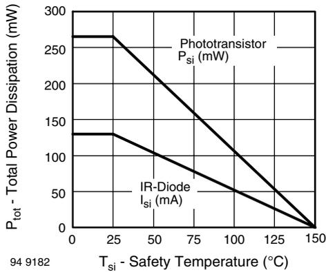
Fig. 1 - Derating Diagram
