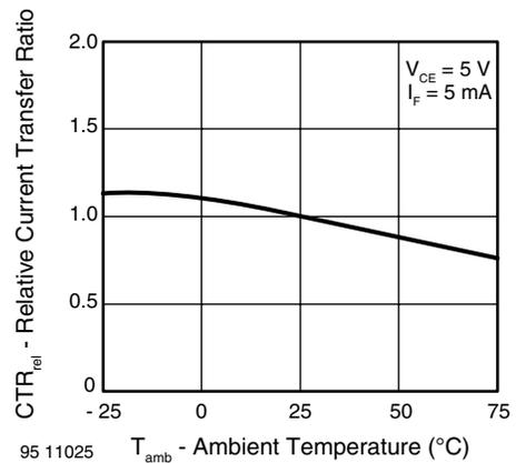
Fig. 8 - Relative Current Transfer Ratio vs. Ambient Temperature
