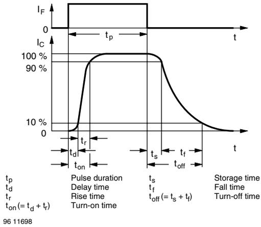
Fig. 5 - Switching Times
