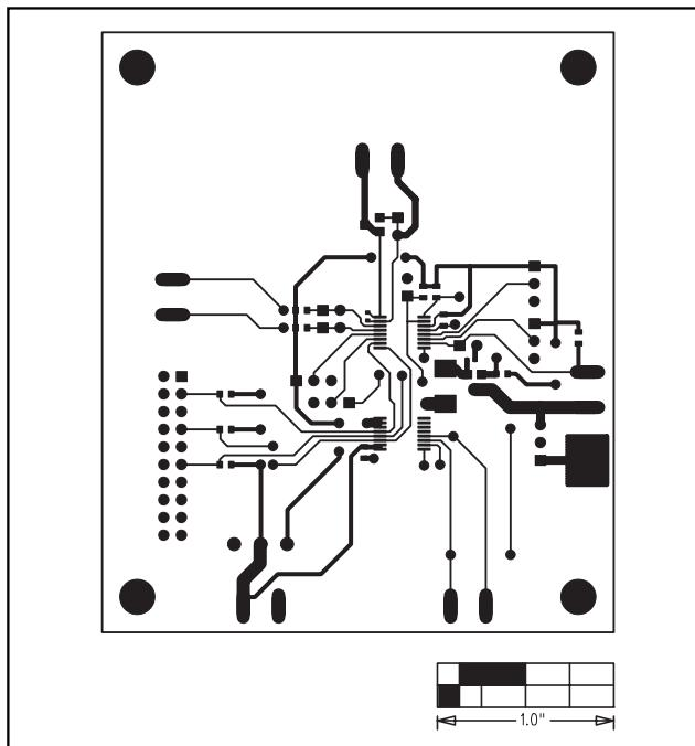
Figure 8. MAX6653 EV Kit PC Board Layout—Component Side
