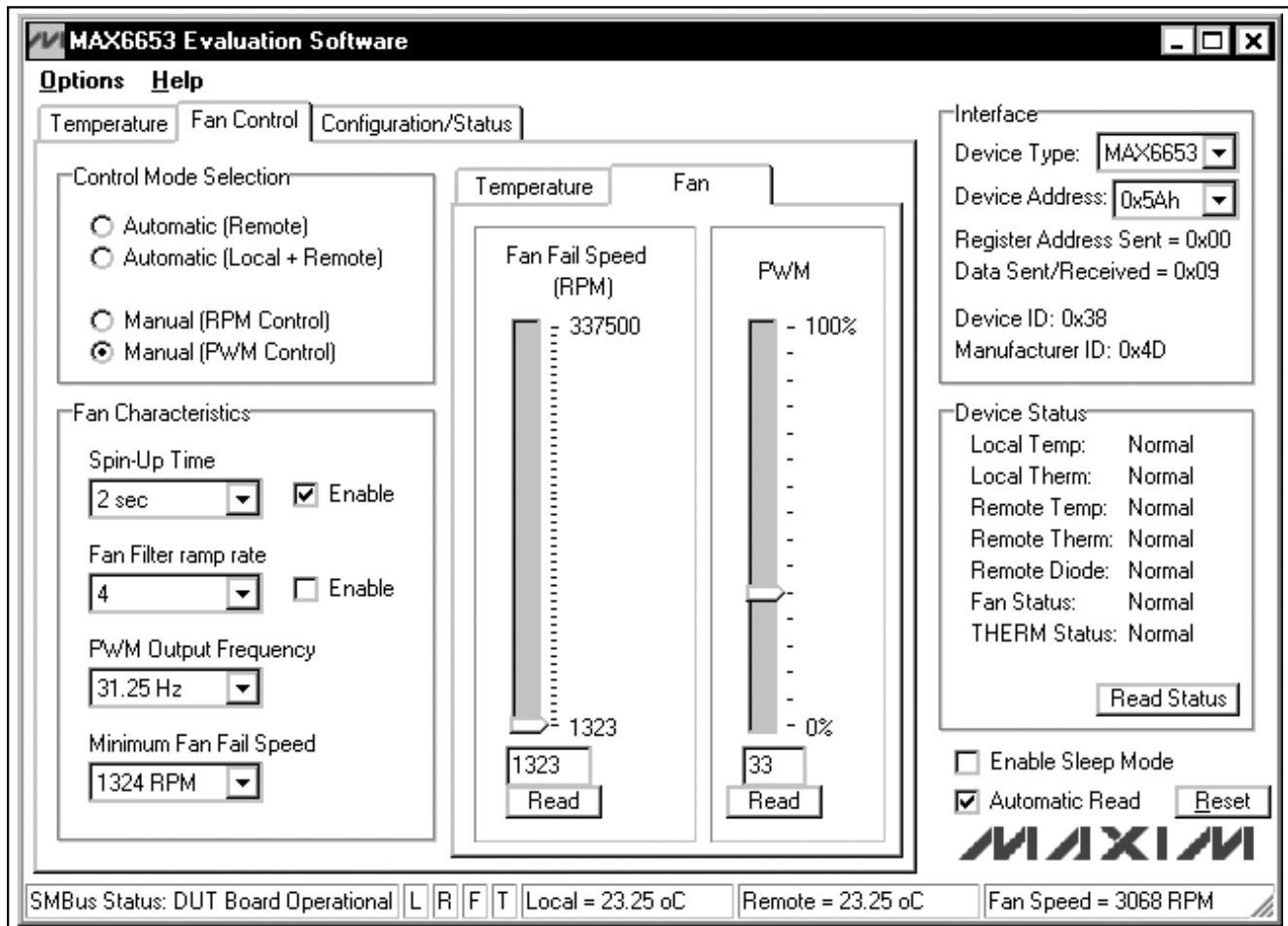
Figure 2b. MAX6653 EV Kit Software Main Window (Fan Control Panel)
