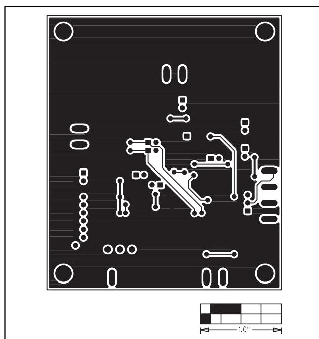
Figure 9. MAX6653 EV Kit PC Board Layout—Solder Side
