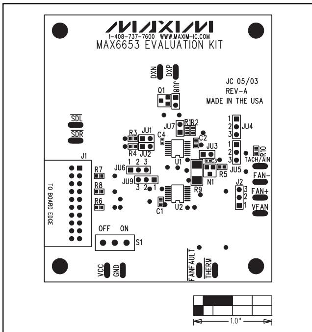
Figure 7. MAX6653 EV Kit Component Placement Guide—Component Side
