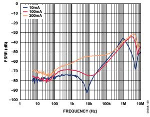
Figure 31. Power Supply Rejection Ratio vs. Frequency,  $V_{OUT} = 1.8 V$ ,  $V_{IN} = 2.3 V$ ,  $V_{RIPPLE} = 50 \text{ mV}$ ,  $C_{OUT} = 1 \mu\text{F}$
