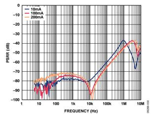
Figure 34. Power Supply Rejection Ratio vs. Frequency,  $V_{OUT} = 1.5 V$ ,  $V_{IN} = 2.5 V$ ,  $V_{RIPPLE} = 50 \text{ mV}$ ,  $C_{OUT} = 1 \mu F$
