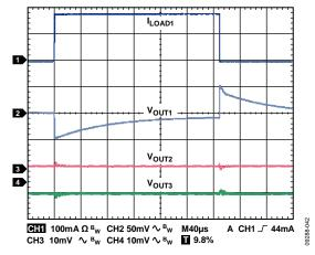
Figure 51. Output Transient Response,  $I_{\text{LOAD1}} = 1 \text{ mA to } 200 \text{ mA}, I_{\text{LOAD2}} = 1 \text{ mA}, I_{\text{LOAD3}} = 1 \text{ mA},$  $CH1 = I_{\text{LOAD1}}, CH2 = V_{\text{OUT1}}, CH3 = V_{\text{OUT2}}, CH4 = V_{\text{OUT3}}$
