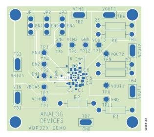
Figure 62. Example of PCB Layout, Top Side
