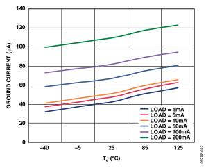
Figure 14. Ground Current vs. Junction Temperature, Single Output Loaded,  $V_{RIPPLE}=50~mV,~C_{OUT}=1~\mu F$
