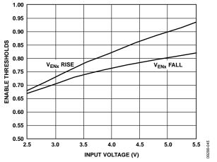
Figure 54. Typical ENx Pins Thresholds vs. Input Voltage
