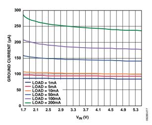
Figure 19. Ground Current vs. Input Voltage, All Outputs Loaded Equally,  $V_{RIPPLE}=50$  mV,  $C_{OUT}=1$   $\mu F$
