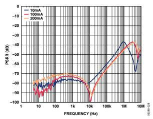
Figure 30. Power Supply Rejection Ratio vs. Frequency,  $V_{OUT} = 1.8 \text{ V}$ ,  $V_{IN} = 2.8 \text{ V}$ ,  $V_{RIPPLE} = 50 \text{ mV}$ ,  $C_{OUT} = 1 \mu F$
