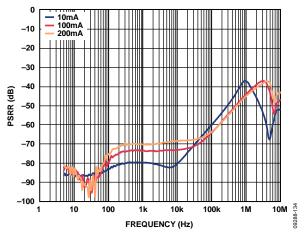
Figure 36. Power Supply Rejection Ratio vs. Frequency,  $V_{OUT} = 1.2 V$ ,  $V_{IN} = 2.2 V$ ,  $V_{RIPPLE} = 50 \text{ mV}$ ,  $C_{OUT} = 1 \mu\text{F}$
