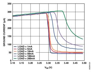
Figure 26. Ground Current vs. Input Voltage (in Dropout),  $V_{OUT1} = 3.3 V$ ,  $V_{RIPPLE} = 50 \text{ mV}$ ,  $C_{OUT} = 1 \mu\text{F}$
