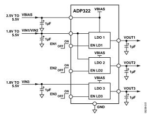
Figure 1. Typical Application Circuit for ADP322
