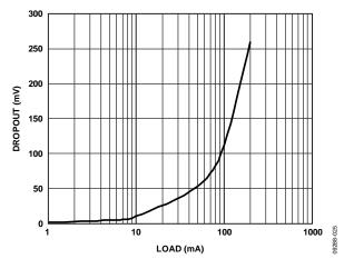
Figure 27. Dropout Voltage vs. Load Current and Output Voltage,  $V_{OUT2}=1.8\,V,\,V_{RIPPLE}=50\,mV,\,C_{OUT}=1\,\mu F$
