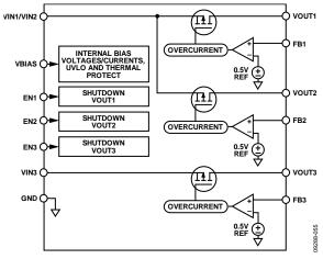
Figure 49. ADP323 Internal Block Diagram
