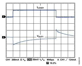
Figure 42. Load Transient Response,  $I_{\text{LOAD1}} = 1 \text{ mA to } 200 \text{ mA}, C_{\text{OUT1}} = 1 \text{ µF}, CH1 = I_{\text{LOAD1}}, CH2 = V_{\text{OUT1}}, V_{\text{RIPPLE}} = 50 \text{ mV}, C_{\text{OUT}} = 1 \text{ µF}$
