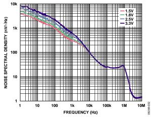
Figure 38. Output Noise Spectral Density,  $V_{\rm IN}$  = 5 V,  $I_{\rm LOAD}$  = 10 mA,  $V_{\rm RIPPLE}$  = 50 mV,  $C_{\rm OUT}$  = 1  $\mu F$
