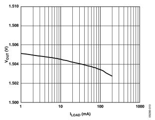
Figure 12. Output Voltage vs. Load Current,  $V_{RIPPLE} = 50 \text{ mV}$ ,  $C_{OUT} = 1 \mu F$
