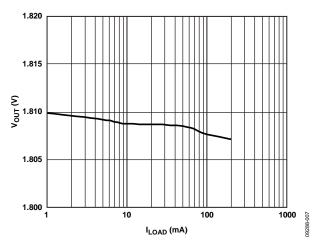
Figure 9. Output Voltage vs. Load Current,  $V_{RIPPLE} = 50 \text{ mV}$ ,  $C_{OUT} = 1 \mu\text{F}$
