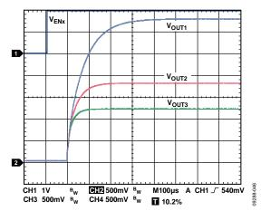
Figure 55. Typical Start-Up Time,  $I_{LOAD1} = I_{LOAD2} = I_{LOAD3} = 100$  mA, CH1 =  $V_{ENx}$  (the Enable Voltage), CH2 =  $V_{OUT1}$ , CH3 =  $V_{OUT2}$ , CH4 =  $V_{OUT3}$
