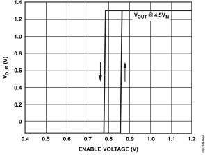
Figure 53. Typical ENx Pin Operation
