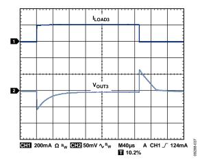
Figure 44. Load Transient Response,  $I_{LOAD3} = 1 \text{ mA to } 200 \text{ mA, } C_{OUT3} = 1 \text{ µF, CH1} = I_{LOAD3},$  $CH2 = V_{OUT3}, V_{RIPPLE} = 50 \text{ mV, } C_{OUT} = 1 \text{ µF}$
