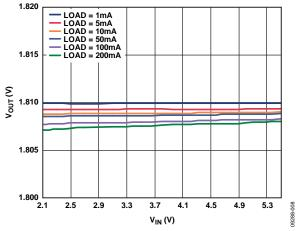
Figure 10. Output Voltage vs. Input Voltage,  $V_{RIPPLE} = 50 \text{ mV}$ ,  $C_{OUT} = 1 \mu\text{F}$
