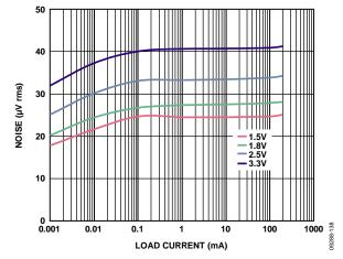
Figure 40. 100 Hz to 100 kHz Output Noise vs. Load Current and Output Voltage,  $V_{\rm IN}$  = 5 V,  $V_{\rm RIPPLE}$  = 50 mV,  $C_{\rm OUT}$  = 1  $\mu F$
