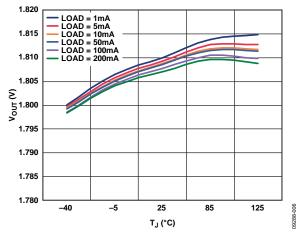
Figure 8. Output Voltage vs. Junction Temperature,  $V_{RIPPLE} = 50 \text{ mV}$ ,  $C_{OUT} = 1 \mu F$
