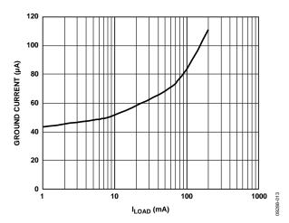
Figure 15. Ground Current vs. Load Current, Single Output Loaded,  $V_{RIPPLE}=50~mV, C_{OUT}=1~\mu F$
