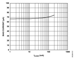
Figure 21. Bias Current vs. Load Current, Single Output Loaded,  $V_{RIPPLE} = 50$  mV,  $C_{OUT} = 1$   $\mu F$
