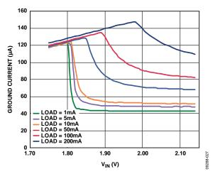
Figure 29. Ground Current vs. Input Voltage (in Dropout),  $V_{OUT2} = 1.8 V$ ,  $V_{RIPPLE} = 50 \text{ mV}$ ,  $C_{OUT} = 1 \mu\text{F}$
