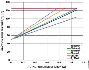
Figure 59. Junction Temperature vs. Total Power Dissipation,  $T_A = 50^{\circ}C$
