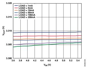
Figure 7. Output Voltage vs. Input Voltage,  $V_{RIPPLE} = 50 \text{ mV}$ ,  $C_{OUT} = 1 \mu F$
