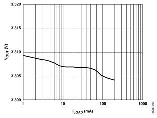
Figure 6. Output Voltage vs. Load Current,  $V_{RIPPLE} = 50 \text{ mV}$ ,  $C_{OUT} = 1 \mu\text{F}$
