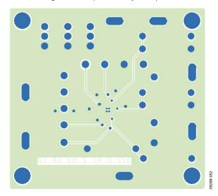
Figure 63. Example of PCB Layout, Bottom Side
