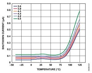
Figure 23. Shutdown Current vs. Temperature at Various Input Voltages,  $V_{RIPPLE}$  = 50 mV,  $C_{OUT}$  = 1  $\mu F$
