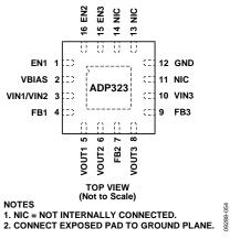
Figure 4. ADP323 Pin Configuration
