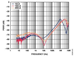
Figure 32. Power Supply Rejection Ratio vs. Frequency,  $V_{\text{OUT}} = 3.3 \text{ V}$ ,  $V_{\text{IN}} = 4.3 \text{ V}$ ,  $V_{\text{RIPPLE}} = 50 \text{ mV}$ ,  $C_{\text{OUT}} = 1 \text{ }\mu\text{F}$
