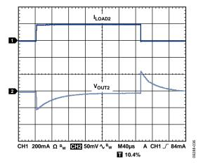
Figure 43. Load Transient Response,  $I_{LOAD2}=1$  mA to 200 mA,  $C_{OUT2}=1$   $\mu F$ ,  $CH1=I_{LOAD2}$ ,  $CH2=V_{OUT2}$ ,  $V_{RIPPLE}=50$  mV,  $C_{OUT}=1$   $\mu F$
