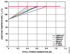
Figure 60. Junction Temperature vs. Total Power Dissipation,  $T_A = 85^{\circ}C$
