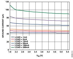
Figure 16. Ground Current vs. Input Voltage, Single Output Loaded,  $V_{RIPPLE}=50~mV,~C_{OUT}=1~\mu F$
