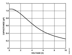
Figure 52. Capacitance vs. Voltage Bias Characteristic
