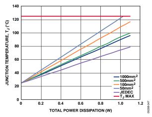
Figure 58. Junction Temperature vs. Total Power Dissipation,  $T_A = 25^{\circ}C$
