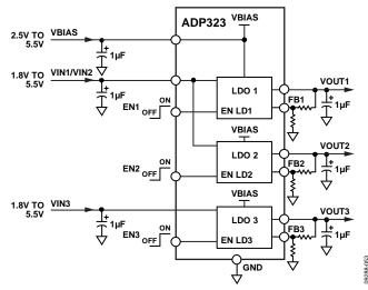
Figure 2. Typical Application Circuit for ADP323
