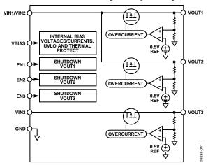
Figure 48. ADP322 Internal Block Diagram
