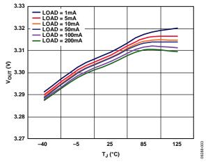
Figure 5. Output Voltage vs. Junction Temperature,  $V_{RIPPLE} = 50 \text{ mV}$ ,  $C_{OUT} = 1 \mu F$
