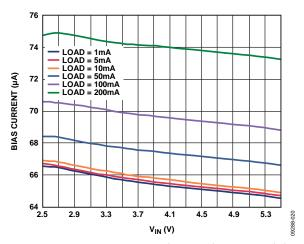
Figure 22. Bias Current vs. Input Voltage, Single Output Loaded,  $V_{RIPPLE} = 50$  mV,  $C_{OUT} = 1$   $\mu F$
