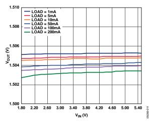
Figure 13. Output Voltage vs. Input Voltage,  $V_{RIPPLE} = 50 \text{ mV}$ ,  $C_{OUT} = 1 \mu\text{F}$
