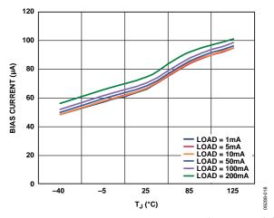
Figure 20. Bias Current vs. Junction Temperature, Single Output Loaded,  $V_{RIPPLE} = 50$  mV,  $C_{OUT} = 1$   $\mu F$
