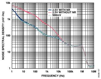
Figure 57. 500 mV and 2.5 V Output Voltage with and Without Noise
