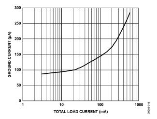
Figure 18. Ground Current vs. Load Current, All Outputs Loaded Equally,  $V_{RIPPLE}$  = 50 mV,  $C_{OUT}$  = 1  $\mu F$
