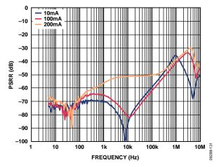
Figure 33. Power Supply Rejection Ratio vs. Frequency,  $V_{OUT} = 3.3 \text{ V}$ ,  $V_{IN} = 3.8 \text{ V}$ ,  $V_{RIPPLE} = 50 \text{ mV}$ ,  $C_{OUT} = 1 \mu\text{F}$
