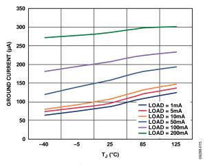
Figure 17. Ground Current vs. Junction Temperature, All Outputs Loaded Equally,  $V_{RIPPLE} = 50 \text{ mV}$ ,  $C_{OUT} = 1 \mu F$
