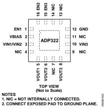
Figure 3. ADP322 Pin Configuration
