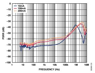
Figure 35. Power Supply Rejection Ratio vs. Frequency,  $V_{\text{OUT}} = 1.5 \text{ V}$ ,  $V_{\text{IN}} = 2.0 \text{ V}$ ,  $V_{\text{RIPPLE}} = 50 \text{ mV}$ ,  $C_{\text{OUT}} = 1 \mu\text{F}$
