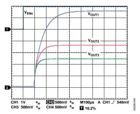
Figure 47. Turn On Response,  $I_{LOAD2} = I_{LOAD2} = I_{LOAD3} = 100$  mA,  $CH1 = V_{ENx}$  (the Enable Voltage),  $CH2 = V_{OUT1}$ ,  $CH3 = V_{OUT2}$ ,  $CH4 = V_{OUT3}$ ,  $V_{RIPPLE} = 50$  mV,  $C_{OUT} = 1$   $\mu F$
