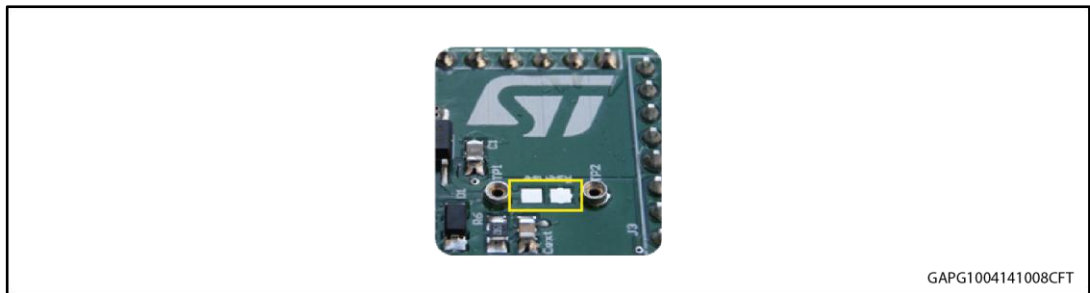
Figure 5: Pads for soldering SMD resistor
