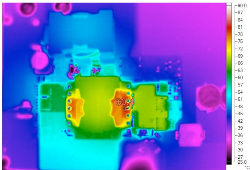
Figure 5. Thermal Map, Front Side at  $48V_{IN}$  and  $5.4A_{OUT}$  ( $T_A = 25^\circ C$ , 200LFM)
