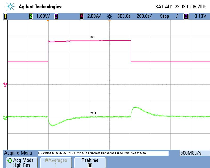
Figure 4. Transient Response Waveform at 48V<sub>IN</sub> and 2.7A to 5.4A to 2.7A<sub>OUT</sub> (2A, 1V, 200μs/DIV)
