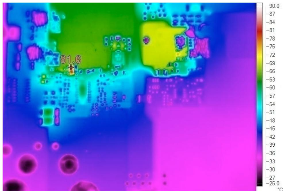
Figure 6. Thermal Map, Back Side at  $48V_{IN}$  and  $5.4A_{OUT}$  ( $T_A = 25^\circ C$ , 200LFM)
