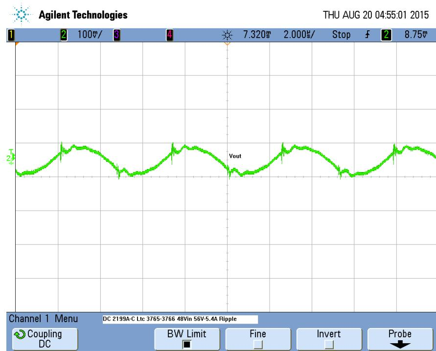
Figure 3. Output Ripple at 48V<sub>IN</sub> and 5.4A<sub>OUT</sub> (100mV, 2μs/DIV, 20MHz)
