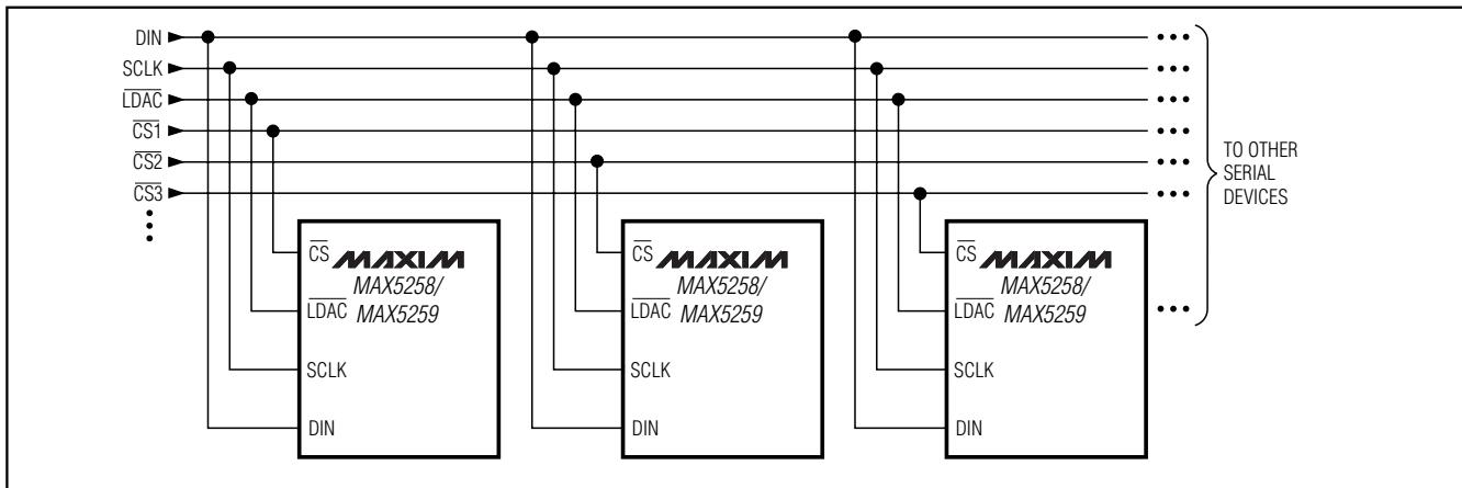
Figure 4. Multiple MAX5258's Sharing One DIN Line. (Simultaneously Update by Strobing LDAC, or Specifically Update by Enabling an Individual CS)
