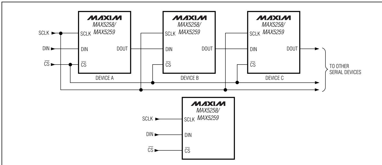
Figure 7. Daisy-Chained or Individual MAX5258s Simultaneously Updated by Bringing CS High (Only Three Wires Are Required)
