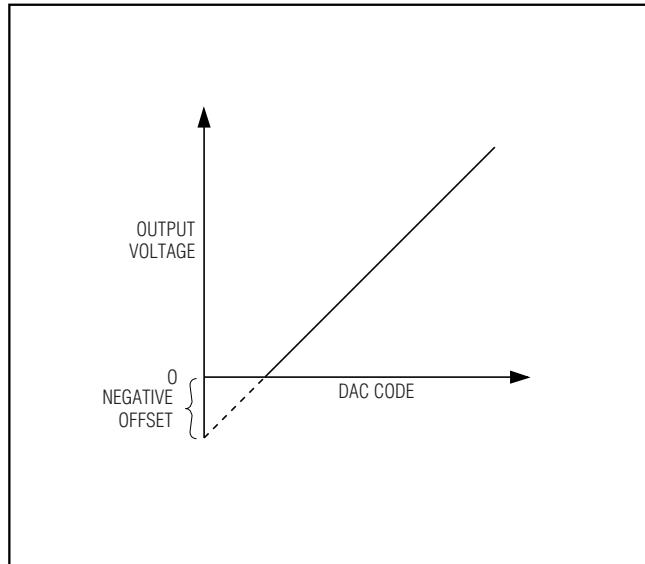
Figure 9. Effect of Negative Offset (Single Supply)
