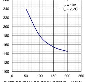
RATE OF CHANGE OF CURRENT :  $di/dt(A/\mu s)$ di/dt-tfr CHARACTERISTICS
