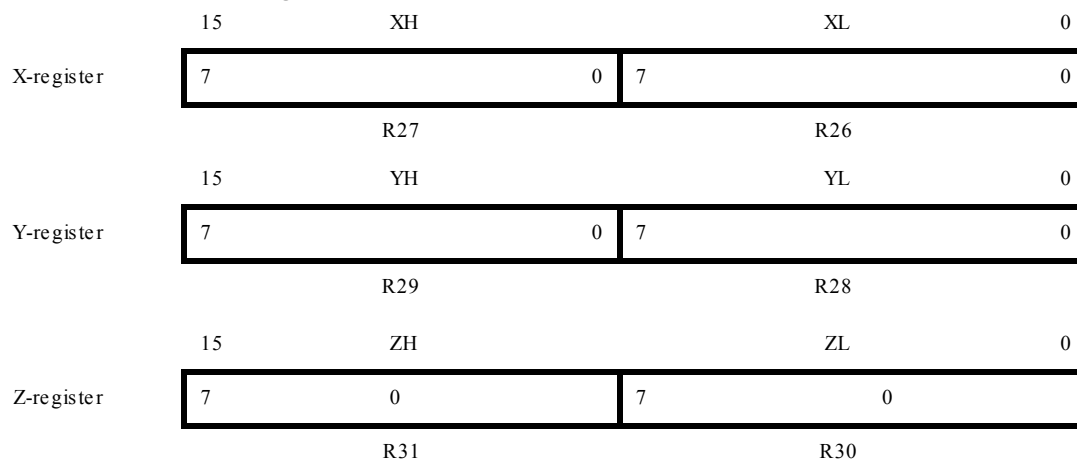
Figure 5-3. The X-, Y-, and Z-registers
