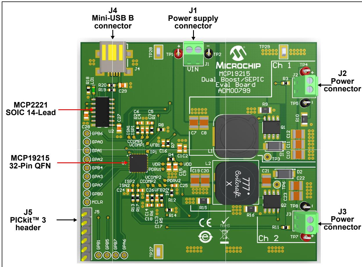
FIGURE 2-1: MCP19215 Dual Boost/SEPIC Evaluation Board – Top View.
