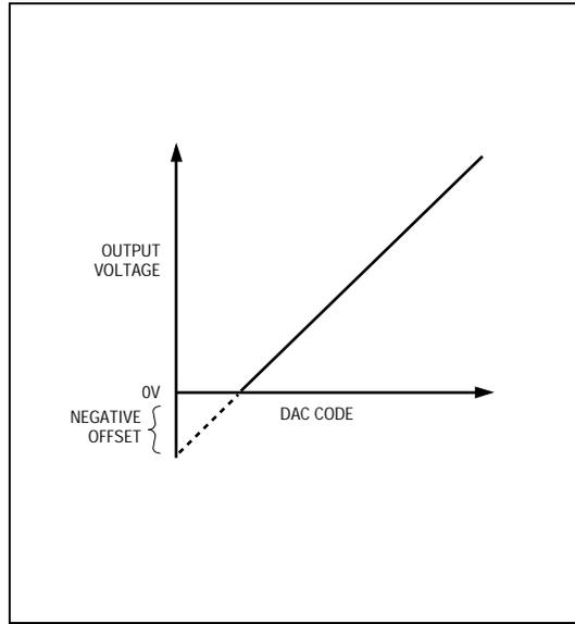
Figure 9. Effect of Negative Offset (Single Supply)
