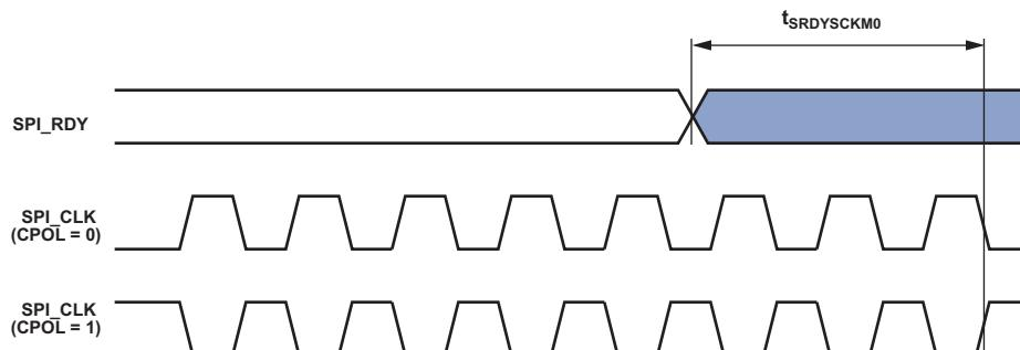
Figure 41. SPI\_RDY Setup Before SPI\_CLK with CPHA = 0
