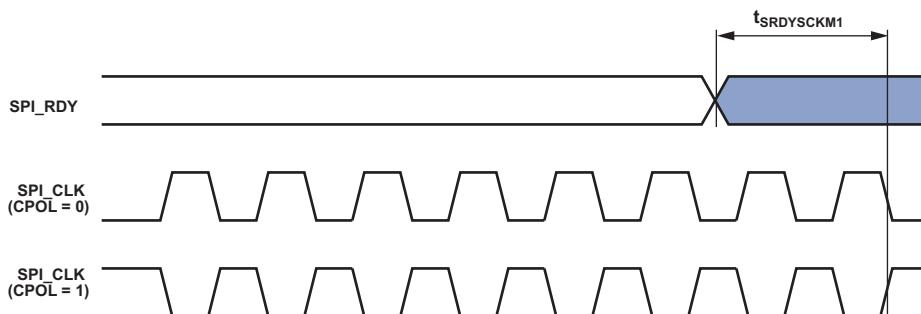
Figure 42. SPI\_RDY Setup Before SPI\_CLK with CPHA = 1
