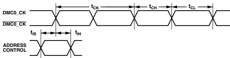
NOTE: CONTROL =  $\overline{\text{DMC0\_CS0}}$ ,  $\overline{\text{DMC0\_CKE}}$ ,  $\overline{\text{DMC0\_RAS}}$ ,  $\overline{\text{DMC0\_CAS}}$ , AND  $\overline{\text{DMC0\_WE}}$ .
