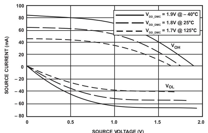
Figure 57. Driver Type C Current (1.8 V  $V_{DD\_DMC}$ )
