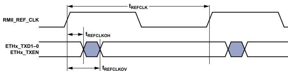
*Figure 51.* 10/100 Ethernet MAC Controller Timing: RMII Transmit Signal
