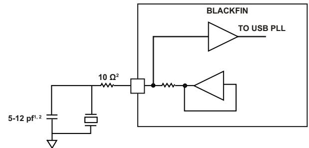
Figure 7. External USB Crystal Connection
