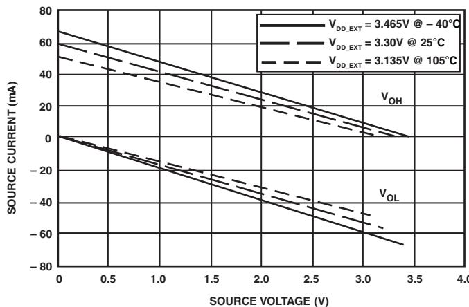
Figure 55. Driver Type A Current (3.3 V  $V_{DD\_EXT}$ )
