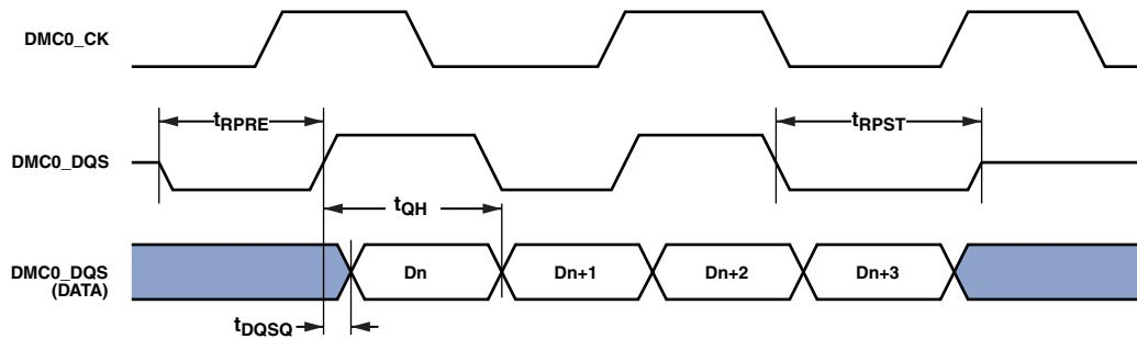
Figure 23. Mobile DDR SDRAM Controller Input AC Timing
