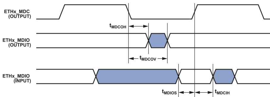
*Figure 52. 10/100 Ethernet MAC Controller Timing: RMII Station Management*
