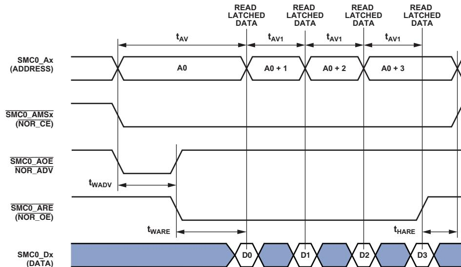
Figure 14. Asynchronous Page Mode Read
