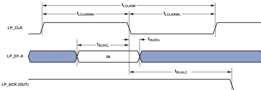
**Figure 29.** Link Ports—Receive
