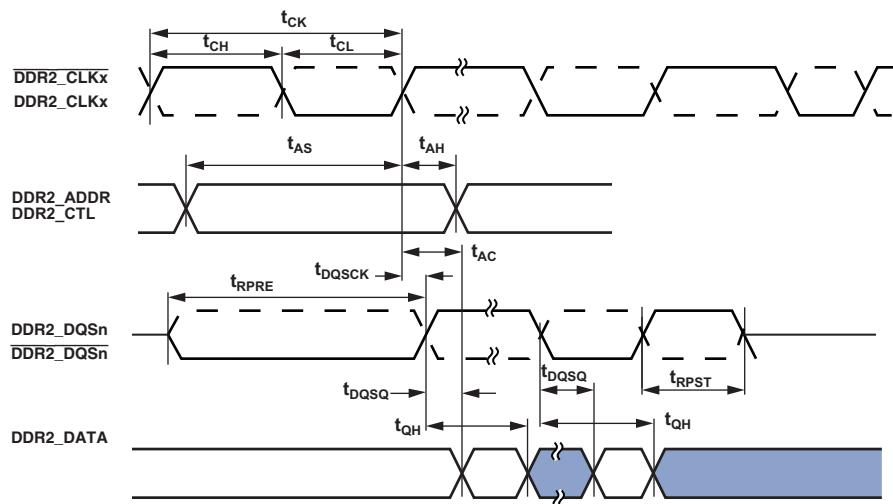
Figure 20. DDR2 SDRAM Controller Input AC Timing
