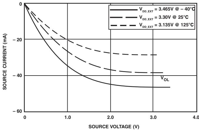
Figure 59. Driver Type D Current ( $3.3 \text{ V } V_{DD\_EXT}$ )
