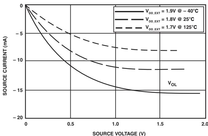
Figure 58. Driver Type D Current ( $1.8 \text{ V } V_{DD\_EXT}$ )
