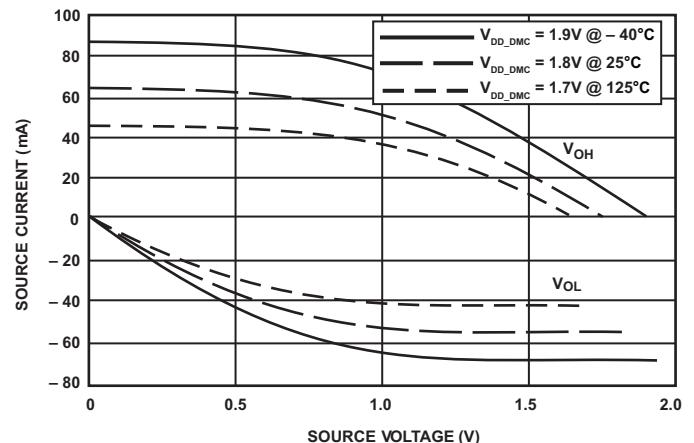
Figure 56. Driver Type B Current (1.8 V  $V_{DD\_DMC}$ )
