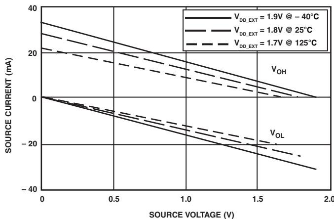
Figure 54. Driver Type A Current (1.8 V  $V_{DD\_EXT}$ )
