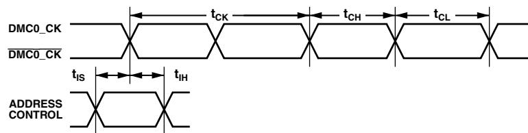
NOTE: CONTROL =  $DMC0\_CS0$ ,  $DMC0\_CKE$ ,  $DMC0\_RAS$ ,  $DMC0\_CAS$ , AND  $DMC0\_WE$ .
