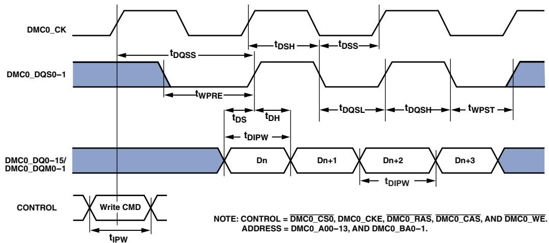
Figure 24. Mobile DDR SDRAM Controller Output AC Timing
