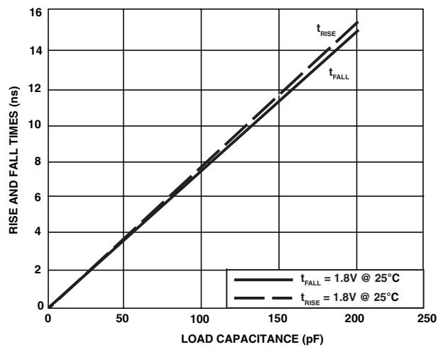
Figure 61. Driver Type A Typical Rise and Fall Times (10%-90%) vs. Load Capacitance ( $V_{DD\_EXT} = 1.8 \text{ V}$ )
