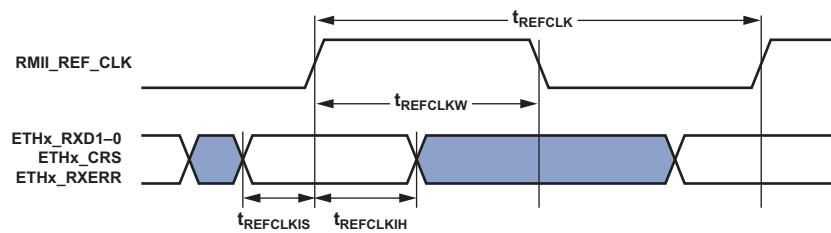
*Figure 50.* 10/100 Ethernet MAC Controller Timing: RMII Receive Signal
