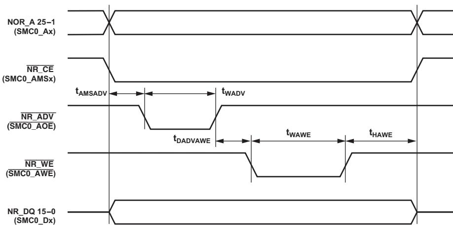
Figure 17. Asynchronous Flash Write
