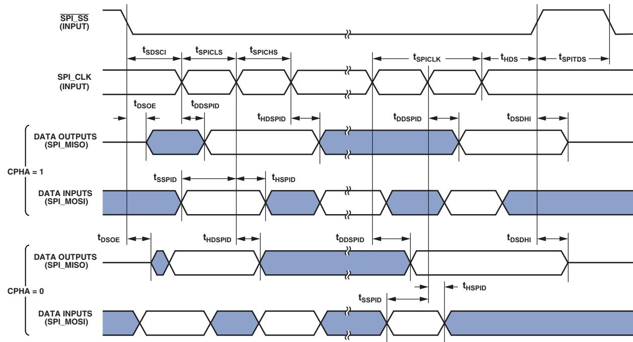
Figure 36. Serial Peripheral Interface (SPI) Port—Slave Timing
