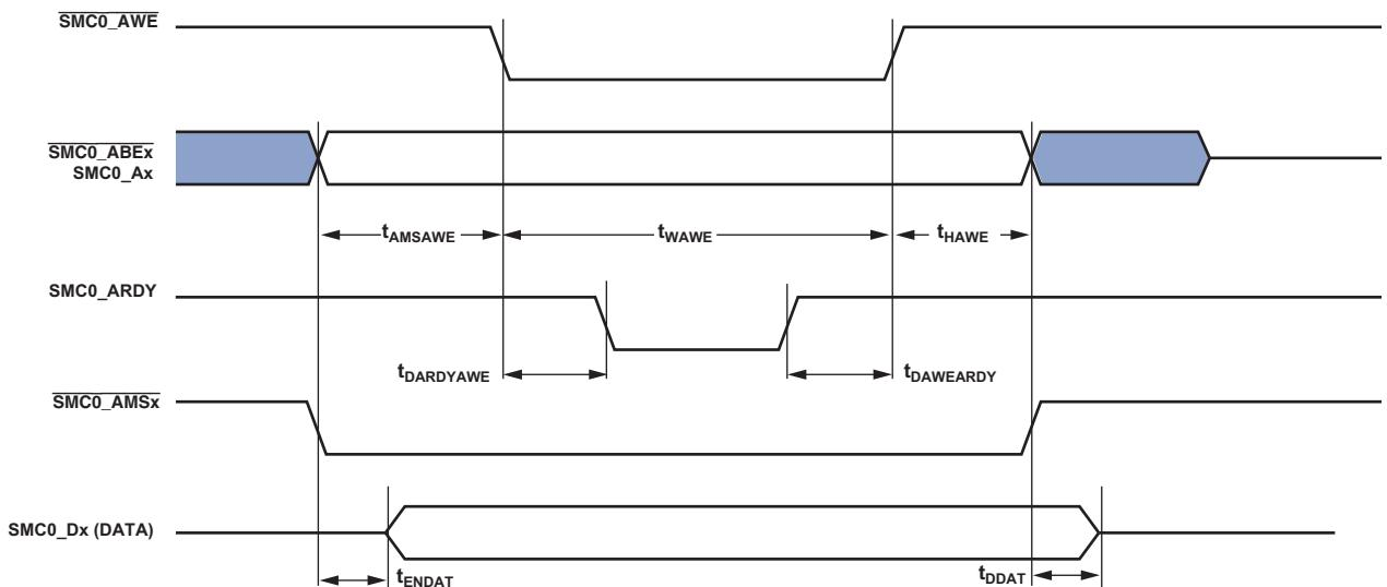
Figure 16. Asynchronous Write
