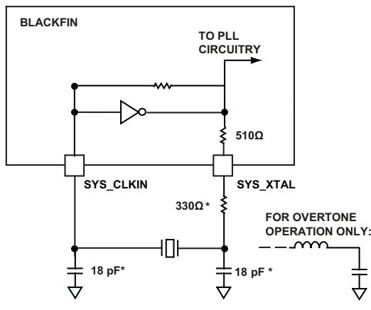
Figure 6. External Crystal Connection
