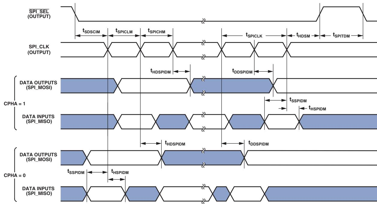
Figure 35. Serial Peripheral Interface (SPI) Port—Master Timing
