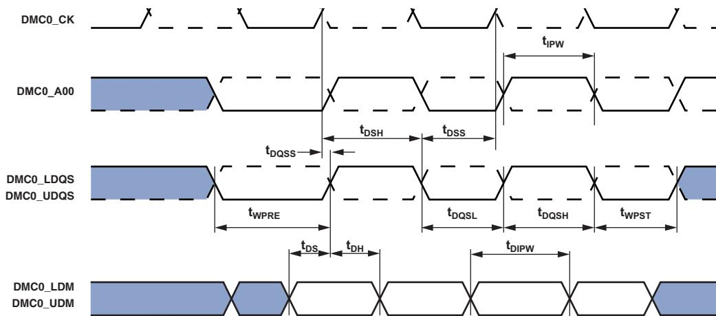
Figure 21. DDR2 SDRAM Controller Output AC Timing
