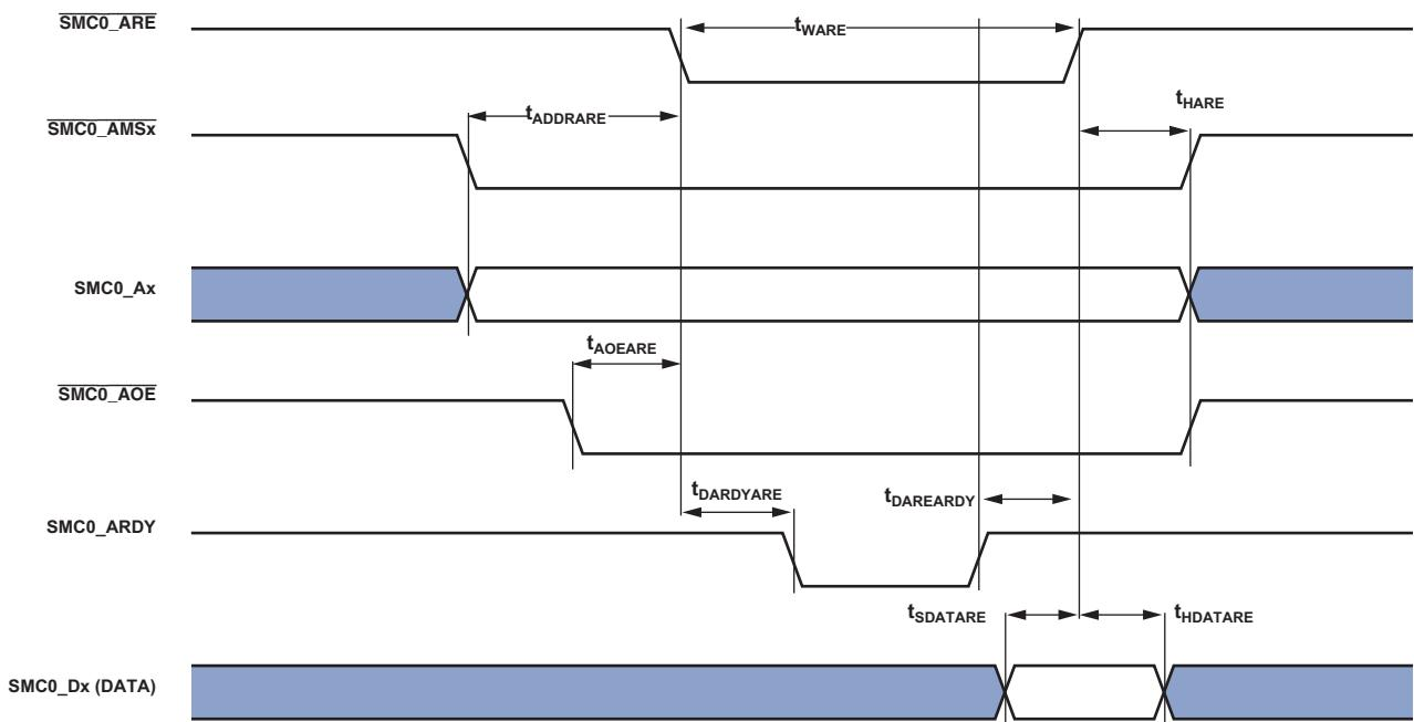
Figure 12. Asynchronous Read
