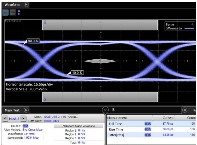
10Gb/s (USB 3.1) Eye Diagram without RClamp3371ZC
