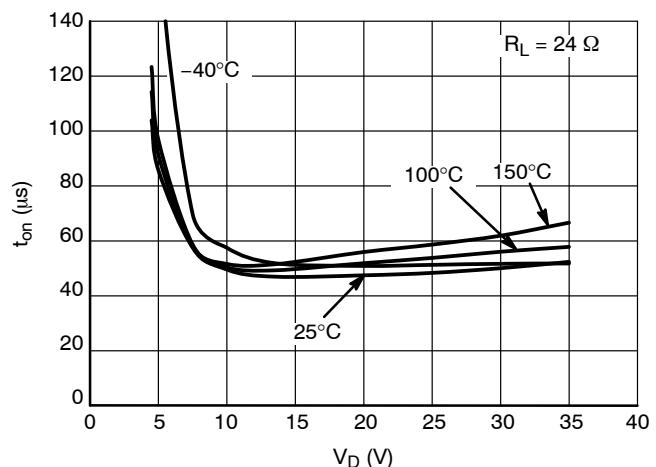
Figure 27. Turn-On Time vs. Supply Voltage
