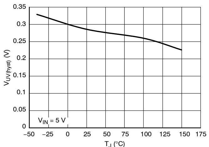
**Figure 17. Under Voltage Shutdown Hysteresis vs. Junction Temperature**
