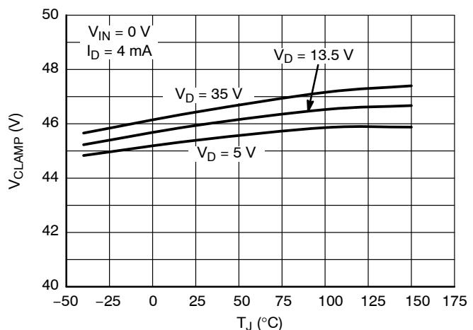
**Figure 21. Output Clamp Voltage vs. Junction Temperature**
