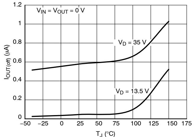
Figure 8. Output Leakage Current vs. Junction Temperature
