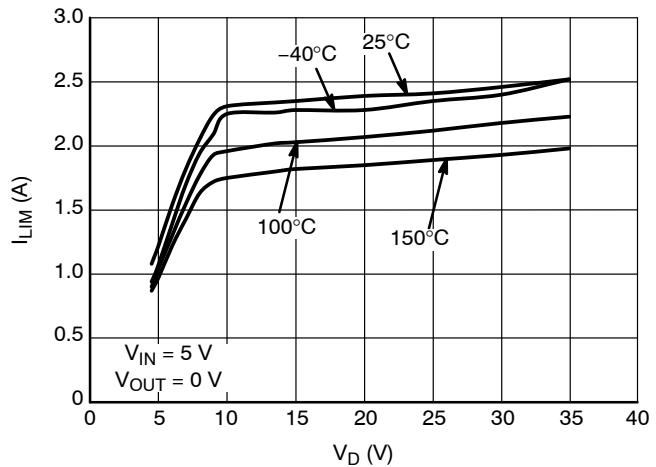
Figure 25. Current Limit vs. Supply Voltage
