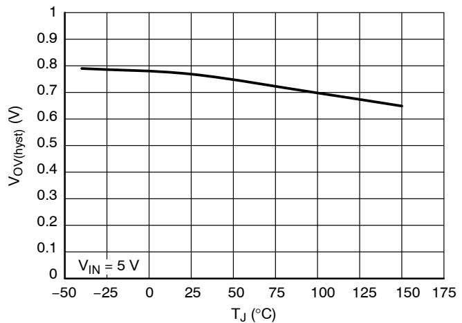
**Figure 19. Over Voltage Shutdown Hysteresis vs. Junction Temperature**
