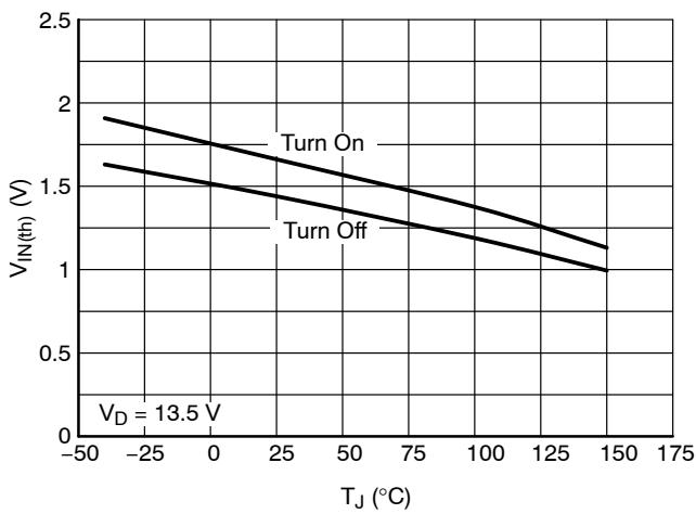
Figure 13. Input Threshold Voltage vs. Junction Temperature
