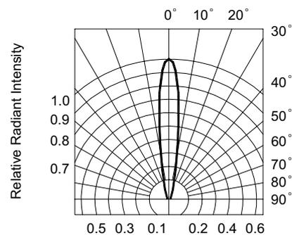
FIG.6 RADIATION DIAGRAM
