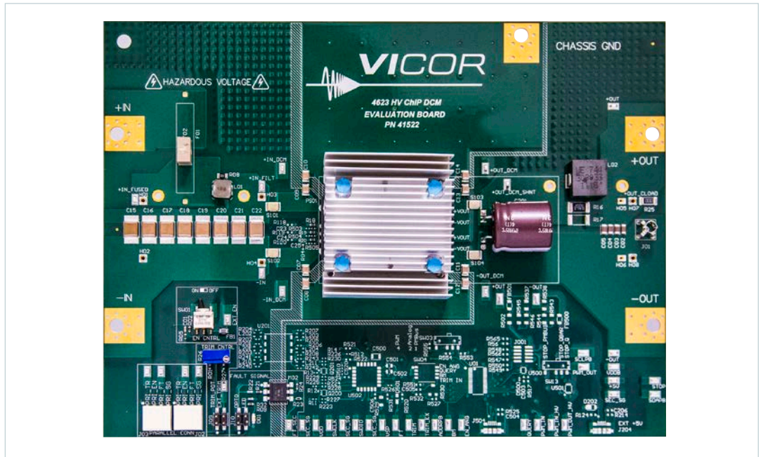
Figure 2 4623 DCM evaluation board photo, top side
