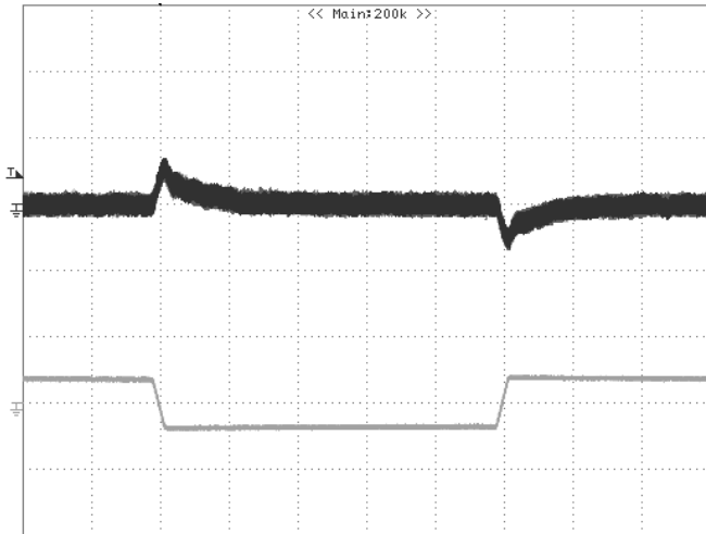
Figure 8: Output voltage response to step-change in load current (75%-50%-75% of I_o , max; di/dt = 0.1A/\mu s ). Load cap: 10\mu F , tantalum capacitor and 1\mu F ceramic capacitor. Top Trace: V_{out} (100mV/div, 200us/div), Bottom Trace: I_{out} (5A/div). Scope measurement should be made using a BNC cable (length shorter than 20 inches). Position the load between 51 mm to 76 mm (2 inches to 3 inches) from the module
