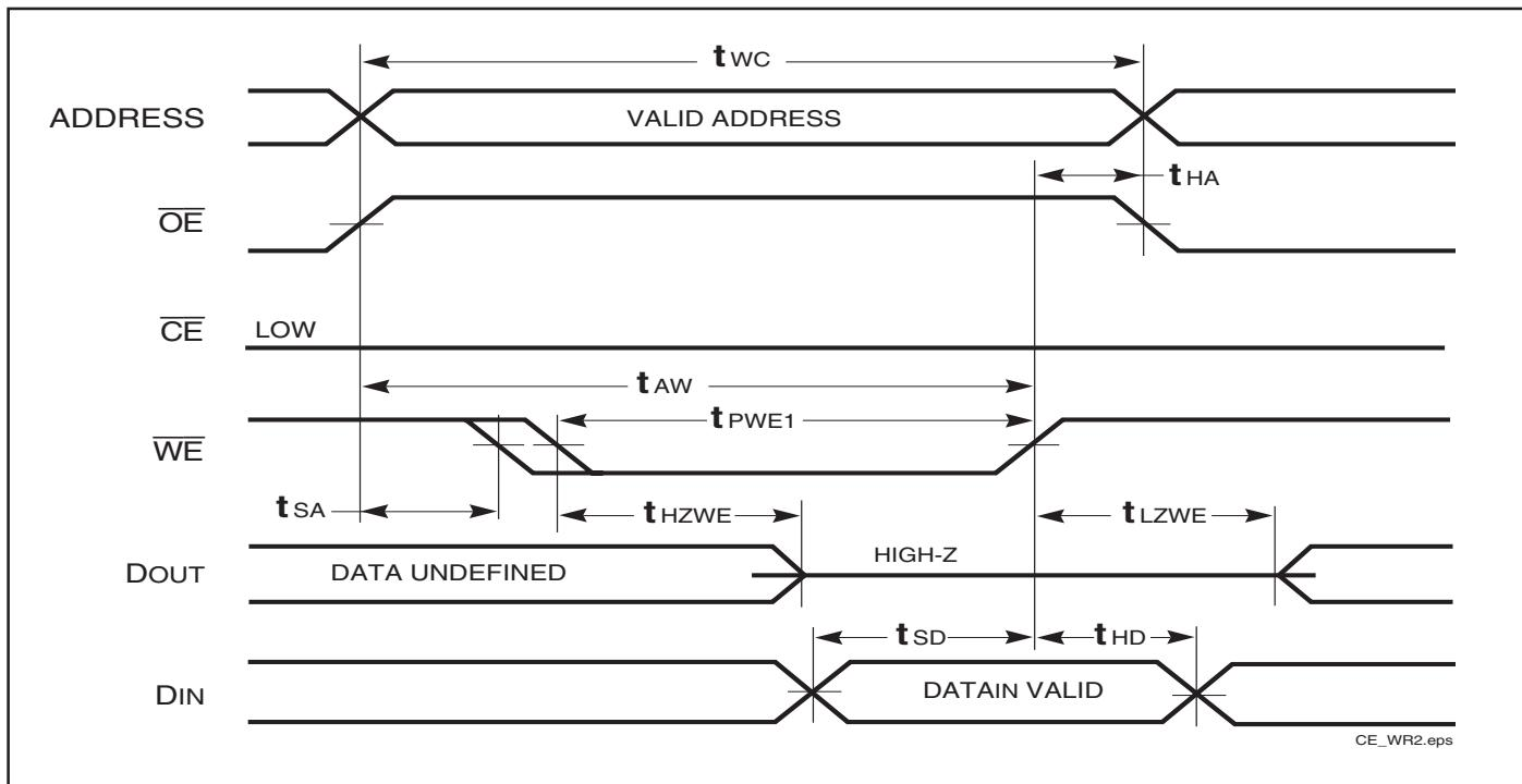
**WRITE CYCLE NO. 3 ( $\overline{OE}$  is LOW During Write Cycle) <sup>(1)</sup>**
