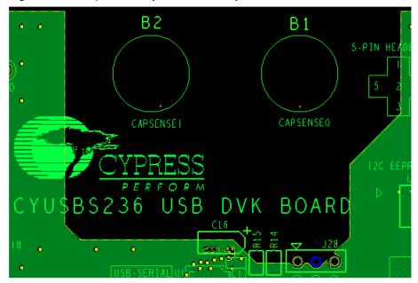
Figure A-11. CapSense Layout - Bottom Layer
