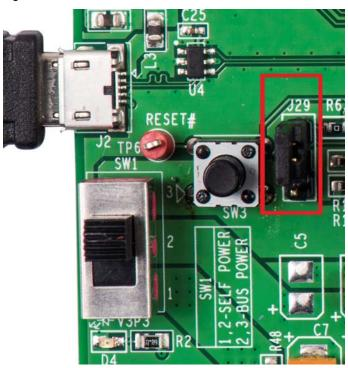
2. Press the reset switch **SW3** on the board. The controller is reinitialized with the new parameters and the board re-enumerates as shown in Figure 3-57.
