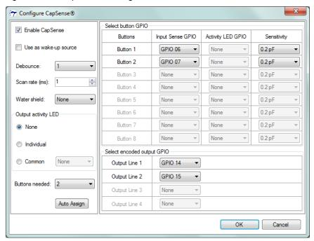
You can configure the following CapSense parameters by using the Cypress USB-Serial Configuration Utility:
