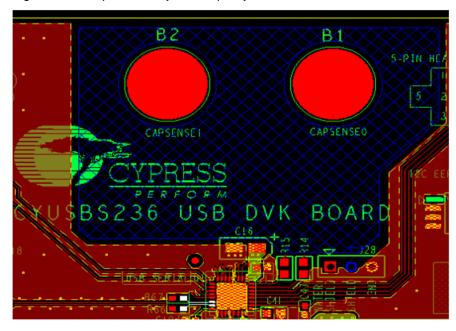
Figure A-9. CapSense Layout - Ground Layer
