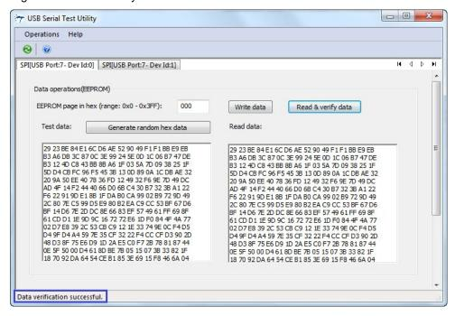
9. To test SCB1 SPI operation, click the **SPI[USB Port:7 - Dev Id:1]** tab, as shown in Figure 3-43. Follow steps 6 to 8 to verify the operation.
