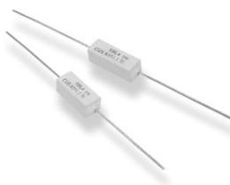
The SBL Series is a low ohmic non-inductive resistor with a low temperature coefficient in a fully insulated ceramic housing. It is ideal for applications in power supply regulation, motor control current monitoring, feedback control loops, overload sensors and radio frequency applications. The solid metal element has welded copper terminals and is encapsulated in a ceramic housing, filled with compressed silica sand.
