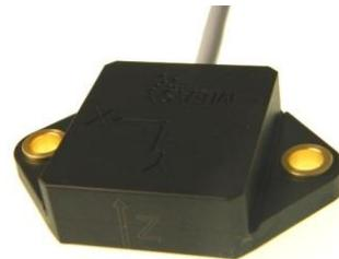
The Model 4020 & 4030 are low noise, signal conditioned DC accelerometers packaged in a durable molded housing. The accelerometers are offered in  $\pm 2g$  &  $\pm 6g$  ranges with a nominal 0-200Hz bandwidth. The model 4020 is a dual axis configuration (X&Y axes) while model 4030 is a triaxial configuration.
