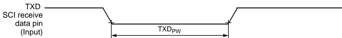
Figure 10-16 TXD Pulse Width
