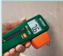
Measures % of Moisture in sheet rock and other building materials using direct pin method. Protective cap snaps onto the side of the housing during use.
