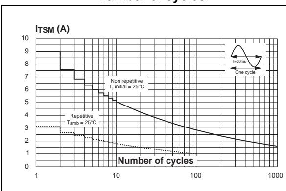
**Figure 4. Non-repetitive surge peak on-state current and corresponding value of  $I^2t$**
