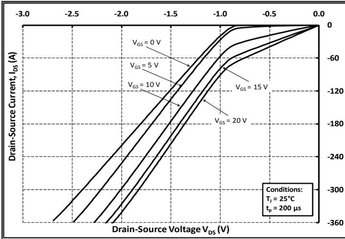
Figure 13. 3<sup>rd</sup> Quadrant Characteristic at 25 °C
