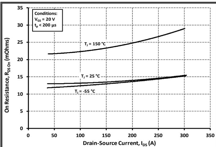
Figure 5. On-Resistance vs. Drain Current For Various Temperatures
