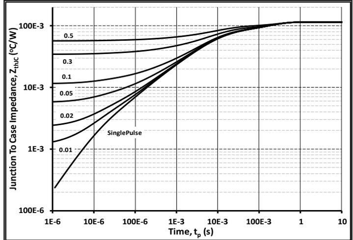
Figure 28. Diode Junction to Case Thermal Impedance
