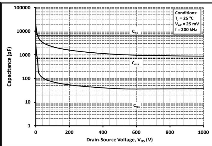
Figure 17. Capacitances vs. Drain-Source Voltage (0 - 1 kV)
