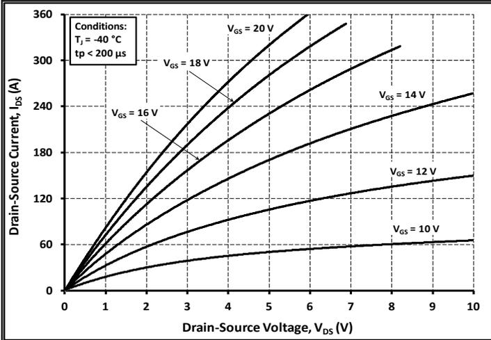
Figure 1. Output Characteristics  $T_j = -40\text{ }^\circ\text{C}$
