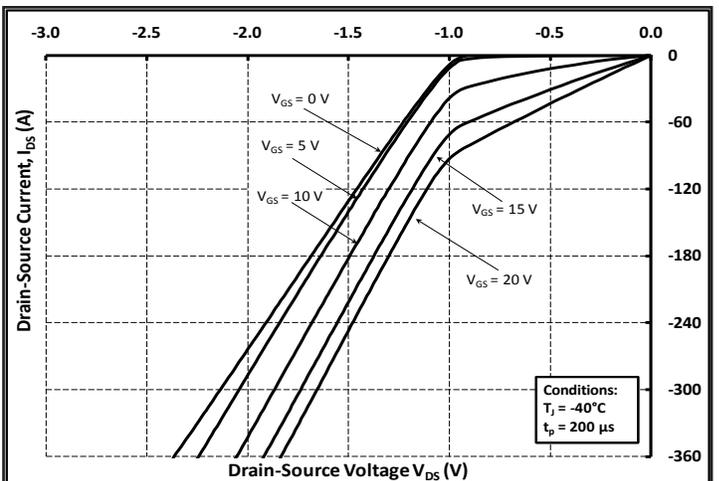
Figure 12. 3<sup>rd</sup> Quadrant Characteristic at -40 °C
