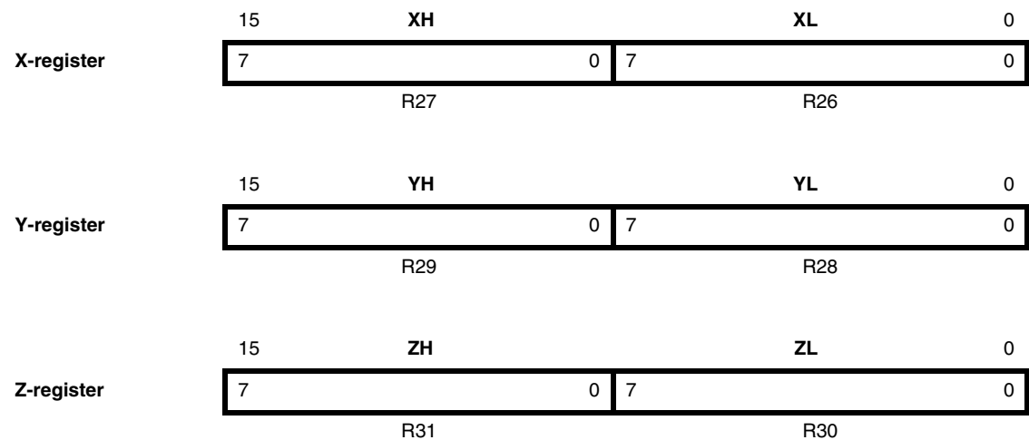
Figure 4-3. The X-, Y-, and Z-registers
