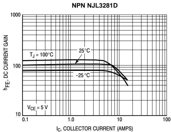
Figure 4. DC Current Gain,  $V_{CE} = 5\text{ V}$
