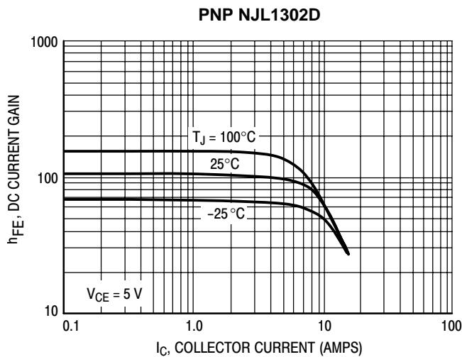
Figure 3. DC Current Gain,  $V_{CE} = 5\text{ V}$
