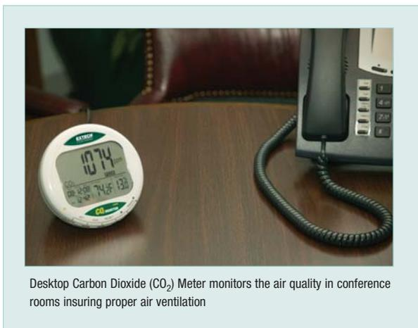
Desktop Carbon Dioxide (CO<sub>2</sub>) Meter monitors the air quality in conference rooms insuring proper air ventilation
