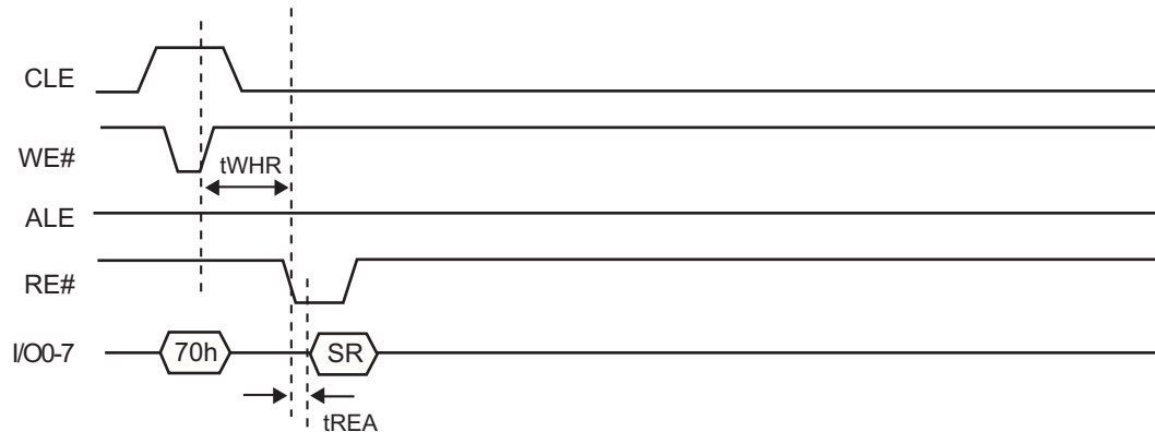
Figure 6.24 Read Status Timing
