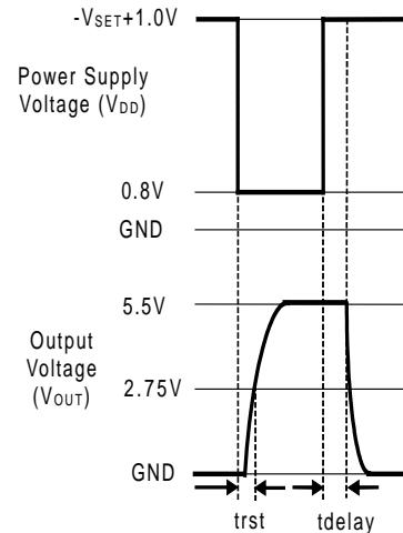
**Figure 10. Nch Open Drain Inverting Output**
