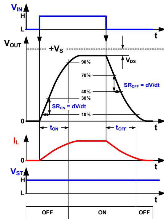
**Waveforms switching a capacitive load:**
