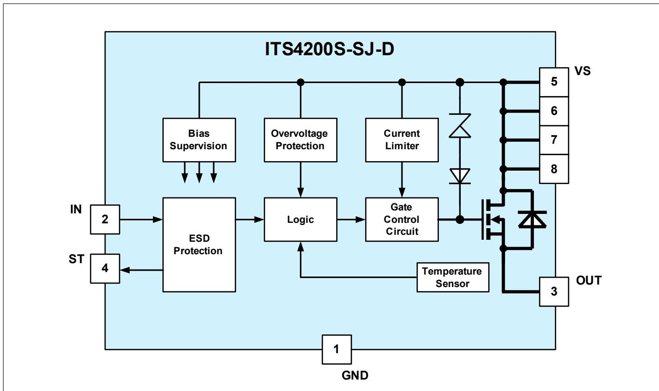
Figure 1 Block diagram
