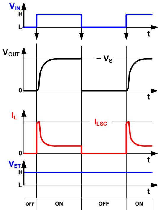
**Waveforms switching an inductive load :**
