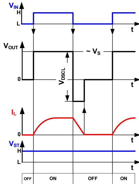
**Figure 6** Typical application waveforms of the ITS4200S-SJ-D
