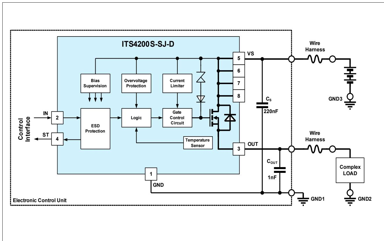
Figure 4 Application Diagram
