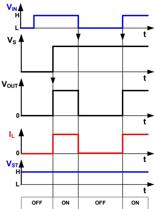
**Waveforms switching a resistive load:**
