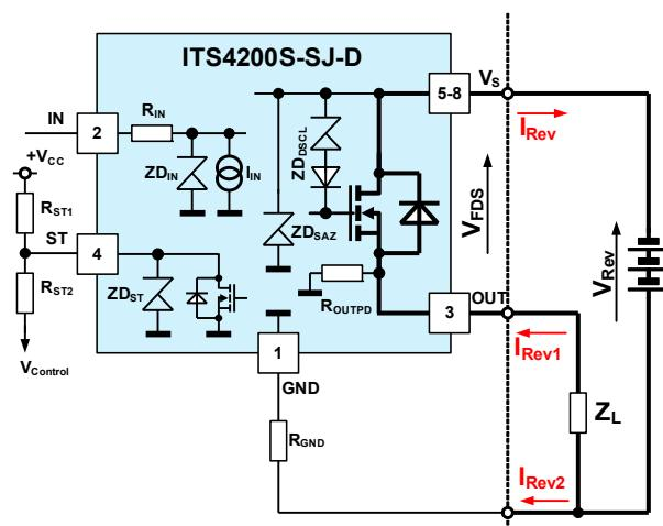
If reverse voltage is applied to the device :
