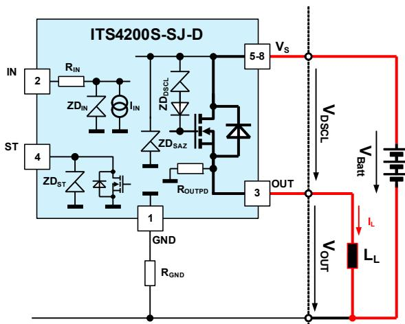
When an inductive load is switched off a current path must be established until the current is sloped down to zero (all energy removed from the inductive load). For that purpose the series combination  $Z_{DSCL}$  is connected between Gate and Drain of the power DMOS acting as an active clamp .
