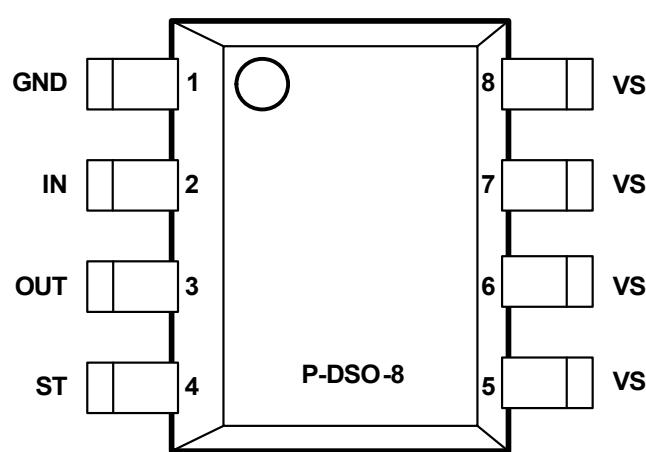
Figure 3 Pin configuration top view, PG-DSO-8
