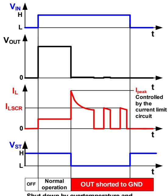
Figure 7 Protective behaviour of the ITS4200S-SJ-D
