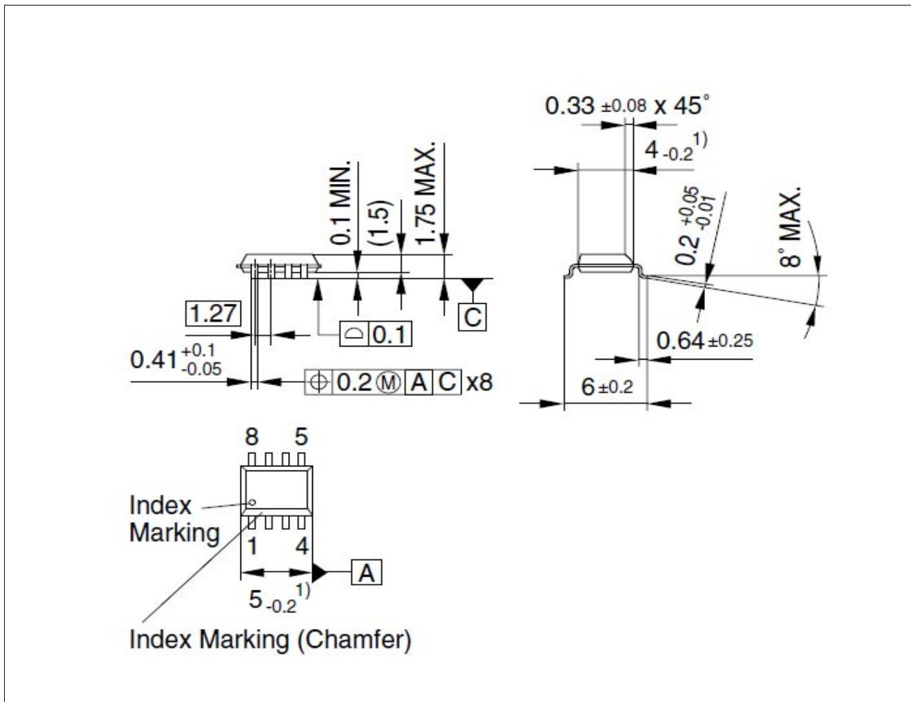
**Figure 8** PG-DSO-8 (Plastic Dual Small Outline Package, RoHS-Compliant)
