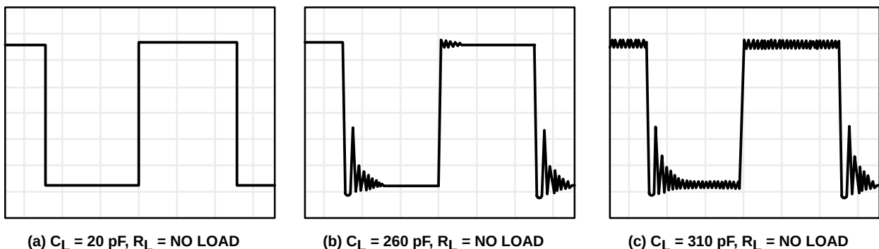
Figure 112. Effect of Capacitive Loads in Low-Bias Mode
