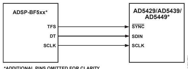
Figure 51. ADSP-BF5xx SPORT-to-AD5429/AD5439/AD5449 Interface
