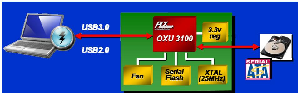
The OXU3100 is a highly integrated device and requires a minimum number of external components. Embedded in the device are a USB 3.0 / 2.0 PHY and device controller, SATA II PHY, internal voltage regulator and Pulse Width Modulators (PWMs) for LED control. The OXU3100 requires only a single external crystal.
