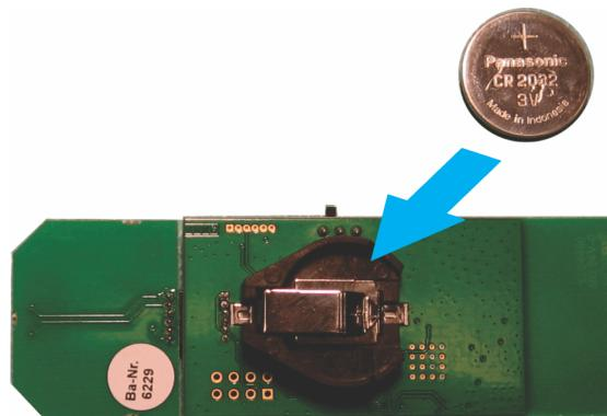
**Figure 5. RF430F5978EVM Battery Assembly**
