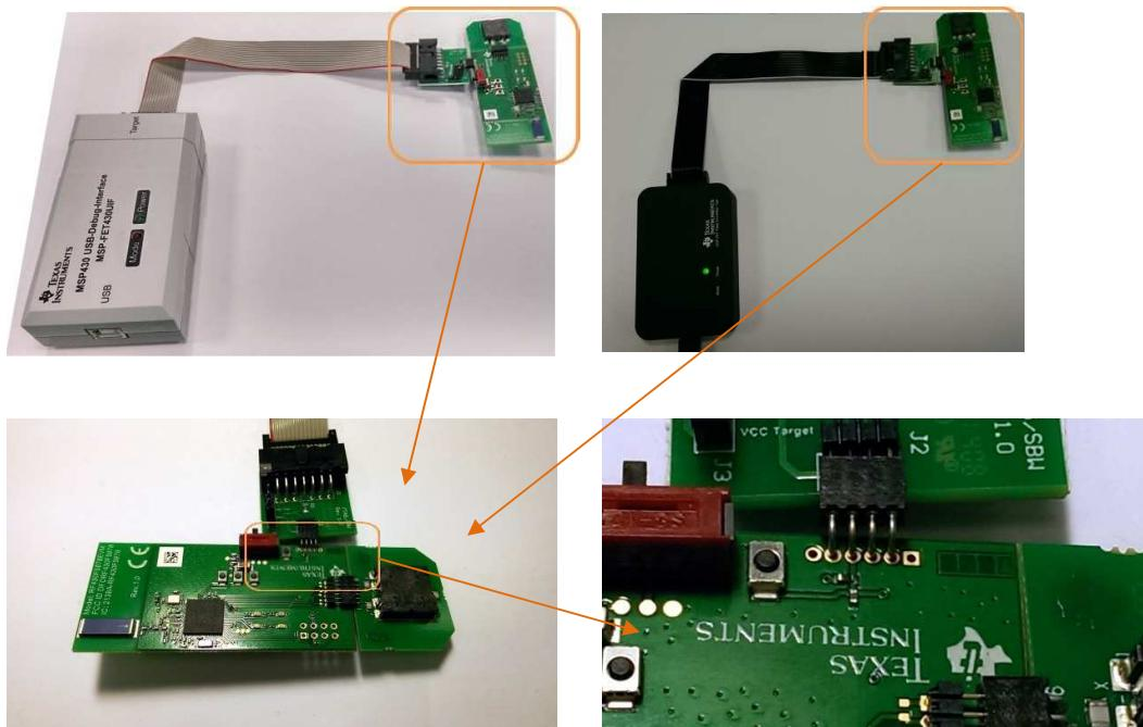
**Figure 21. Connect FET Tool to RF430F5978EVM Module**
