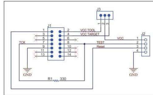
Figure 17. JTAG/SBW Adapter Schematic
