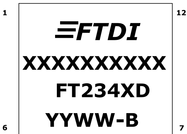
Figure 9.2 DFN-12 Package Markings
