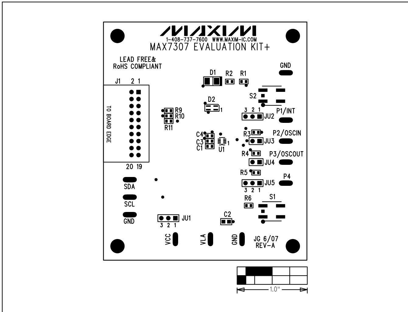
Figure 4. MAX7307 EV Kit Component Placement Guide—Component Side
