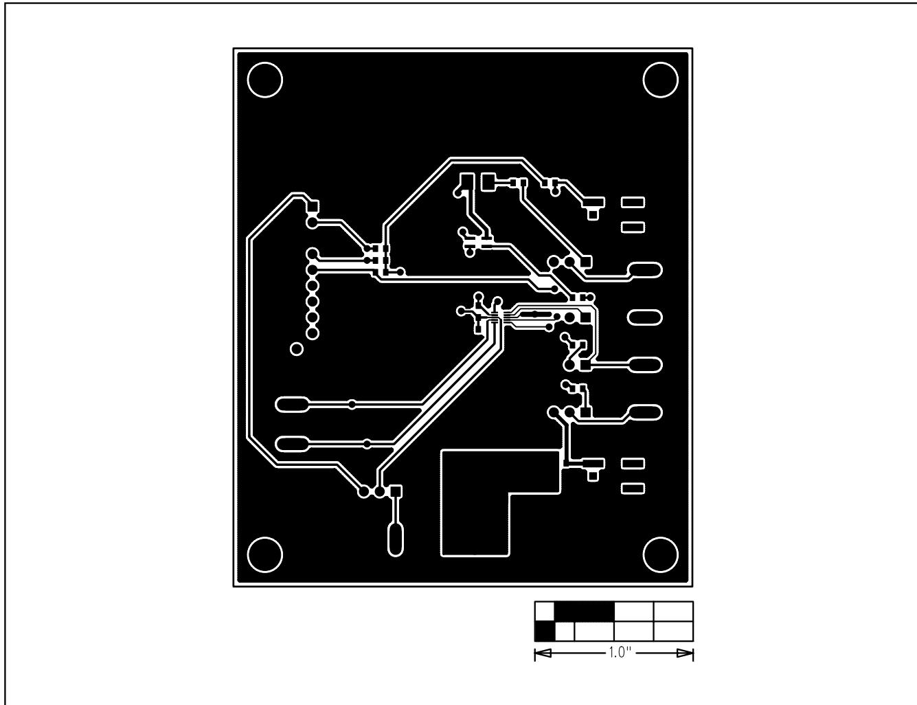
Figure 5. MAX7307 EV Kit PCB Layout—Component Side
