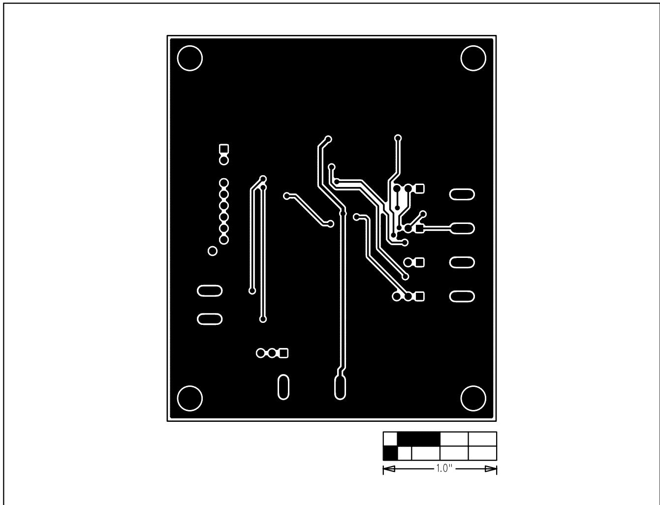
Figure 6. MAX7307 EV Kit PCB Layout—Solder Side
