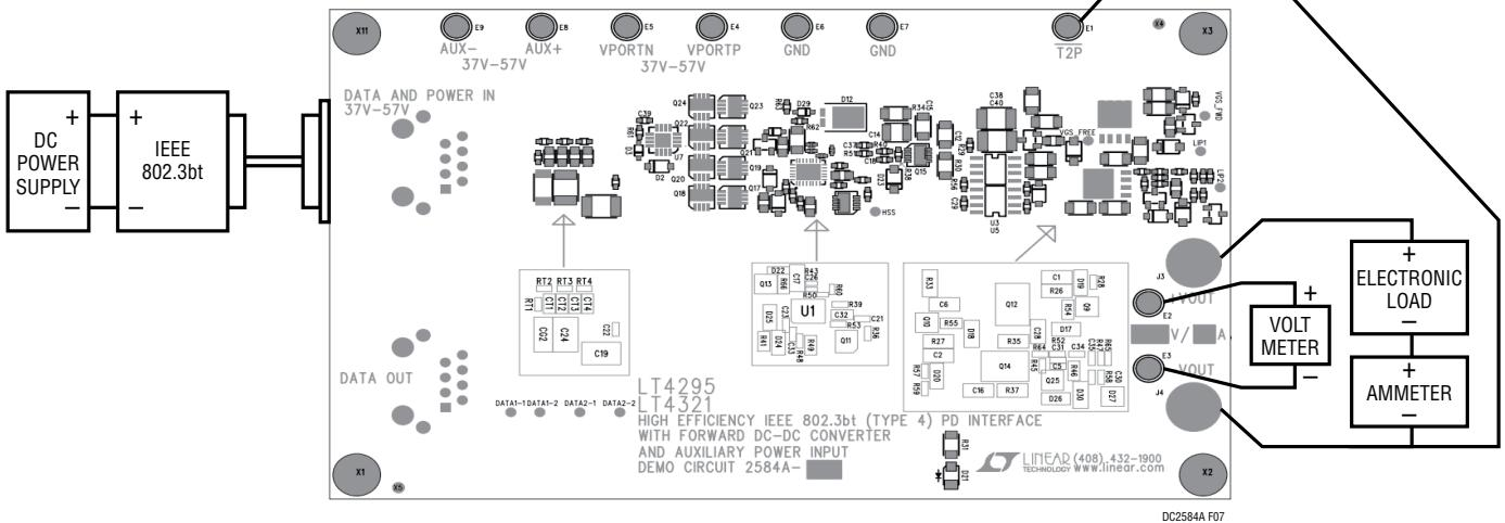
**Figure 7. Setup Diagram for PoE Input**
