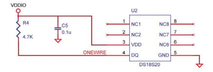
Figure 3-4 1-Wire Temperature Sensor Connectivity
