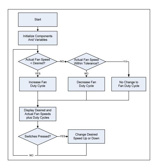
Figure 4-16 Example1 Firmware Flowchart
