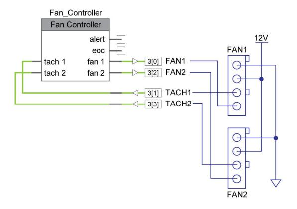
Figure 3-6 Fan Connectivity to PSoC
