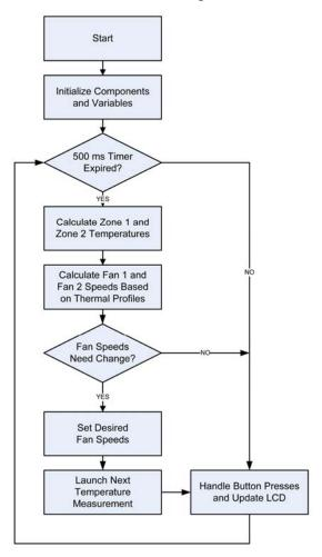
Figure 4-26 Thermal Manager Flowchart
