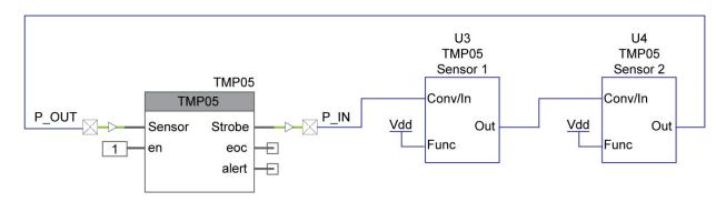
Figure 3-2 TMP05 Temperature Sensor Connectivity
