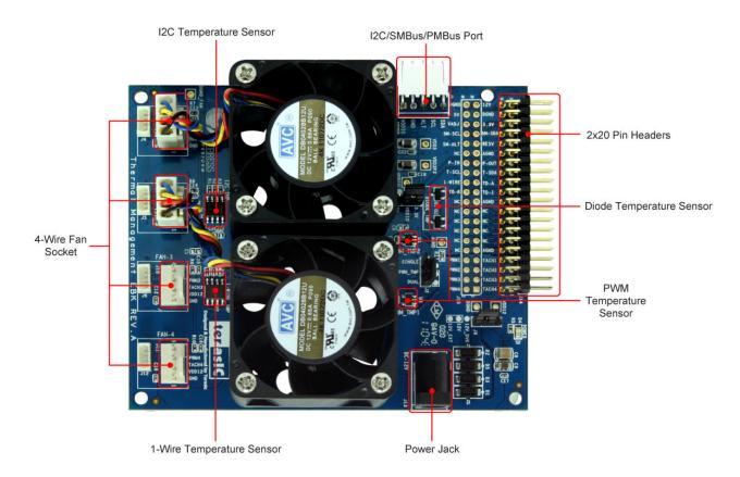
Figure 3-1 TME Hardware Components
