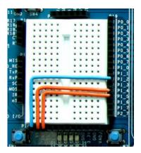
Figure 4-2 CY8CKIT-001 PSoC DVK Breadboard
