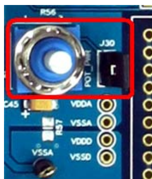
Figure 4-7 CY8CKIT-030 PSoC 3 DVK Potentiometer Power
