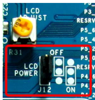
Figure 4-4 CY8CKIT-001 PSoC DVK LCD Power Jumper
