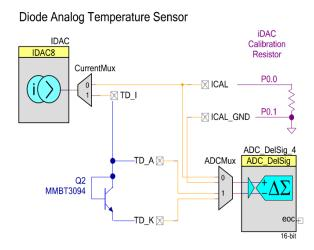
Figure 3-5 Diode Analog Temperature Sensor Connectivity
