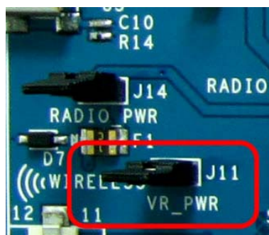
Figure 4-5 CY8CKIT-001 PSoC DVK VR_POWER Jumper
