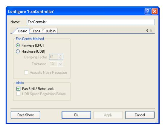
Figure 4-14 Example1 Fan Controller Customizer – Basic Tab
