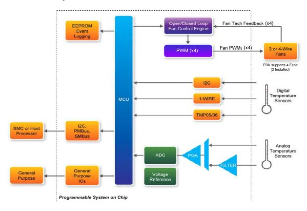
Figure 2-3 Thermal Management Functional Block Diagram
