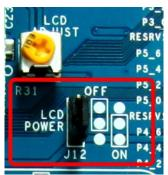
Figure 4-4 CY8CKIT-001 PSoC DVK LCD Power Jumper
