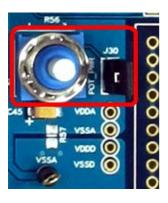
Figure 4-7 CY8CKIT-030 PSoC 3 DVK Potentiometer Power
