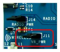
Figure 4-5 CY8CKIT-001 PSoC DVK VR\_POWER Jumper
