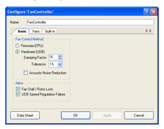
Figure 4-19 Example 2 Fan Controller Customizer – Basic Tab
