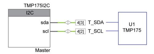
Figure 3-3 I2C Temperature Sensor Connectivity
