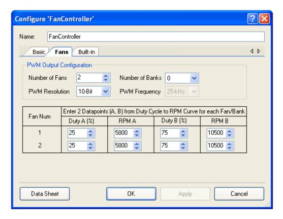
Figure 4-15 Example1 Fan Controller Customizer – Fans Tab
