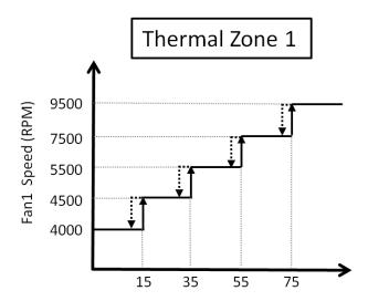
Figure 4-21 Example3 - Zone 1 Thermal Profile
